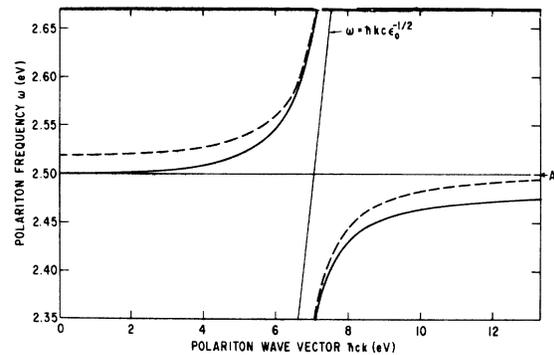
FIG. 2. Dipole and quadrupole polariton frequencies  $\omega$  vs wave vector  $\hbar ck$ , for a single level with  $E = 2.50$  eV,  $|g|^2 = 0.75$  eV<sup>3</sup>, and  $\epsilon_0 = 8$ . Broken line: dipole; solid line: quadrupole. "A" indicates the energy level  $E$ .
