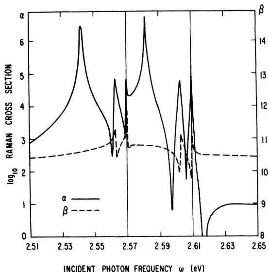
FIG. 13.  $\log_{10}$  Raman cross section vs photon frequency  $\omega$ , in the presence of damping. Solid line: allowed; dashed line: forbidden. CdS parameters are employed. Discrete state  $\Gamma$  is taken as 0.0005, while  $\Gamma \rightarrow +0$  is employed for the continuum. Peaks associated with  $E_1$  and  $E_1 + \omega_0$  are evident (cf. Fig. 4).
