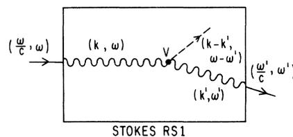
FIG. 1. Schematic of Stokes RS1 scattering by polaritons. An incident photon with (wave vector, frequency)  $= (\omega/c, \omega)$ , represented by a straight line, excites a polariton  $(k, \omega)$  in the crystal, represented by a wavy line. The polariton scatters via the interaction  $V$ , producing a phonon  $(k-k', \omega-\omega')$ , represented by a dashed line. The scattered polariton  $(k', \omega')$  finally emerges as the photon  $(\omega'/c, \omega')$ .
