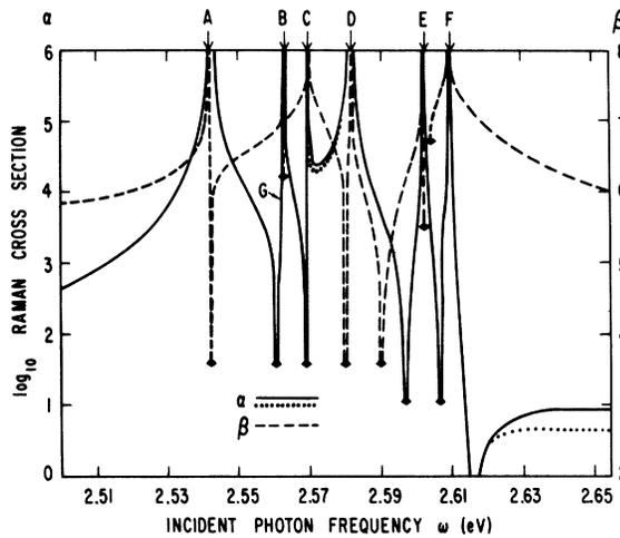
FIG. 9.  $\log_{10}$  of allowed cross section vs photon frequency  $\omega$  for various values of  $g_c/g_1$  and  $E_M$ . Solid line:  $g_c/g_1 = (g_c/g_1)_0$ ,  $E_M = (E_M)_0$  (CdS values); dashed line:  $g_c/g_1 = 10(g_c/g_1)_0$ . Dashed lines indicate departures from CdS results when  $E_M = 10(E_M)_0$ . A–F have the meanings specified in Fig. 7. A nearly vertical dashed line, omitted for clarity, should pass just to the right of point G.
