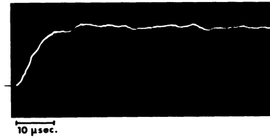
FIG. 6. Pyroelectric detector signal corresponding to the detection of a 1\text{-}\mu\text{W} 20-nsec ir pulse emitted at \lambda = 34.6 \mu .
