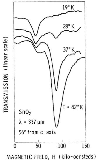
FIG. 1. Transmission through  $\text{SnO}_2$  at several temperatures vs magnetic field. An HCN laser provided continuous-wave monochromatic radiation at a wavelength of  $337 \mu\text{m}$ . The high-field resonance is a true electron cyclotron resonance; the low-field absorption line has not been identified.
