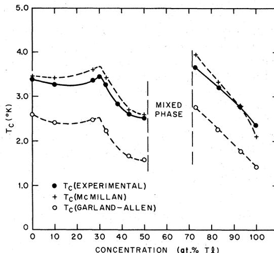
FIG. 1. Comparison of the experimentally measured transition temperatures with those obtained from the theoretical expressions of McMillan (using  $\langle\omega\rangle$  as defined in the text) and of Garland and Allen. This is a revised Fig. 7.
