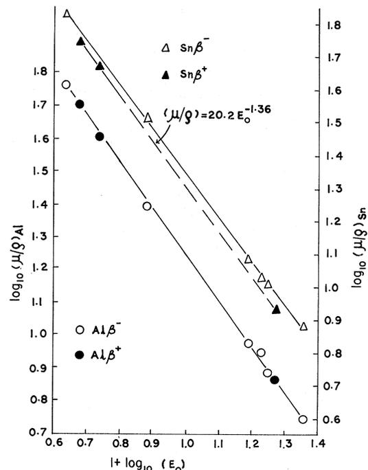
FIG. 2. Experimentally determined values of  $\log_{10} \mu/\rho$  ( $\text{cm}^2 \text{g}^{-1}$ ) plotted as a function of  $\log_{10} E_0$  (MeV). The solid lines are the least-squares straight-lines fits for negative  $\beta$ -particle sources.
