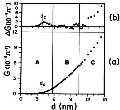
FIG. 6. (a) The conductance  $G$  of the film vs film thickness  $d$ . (b)  $\Delta G = (G - G_{\text{fit}})$  vs film thickness  $d$ .
