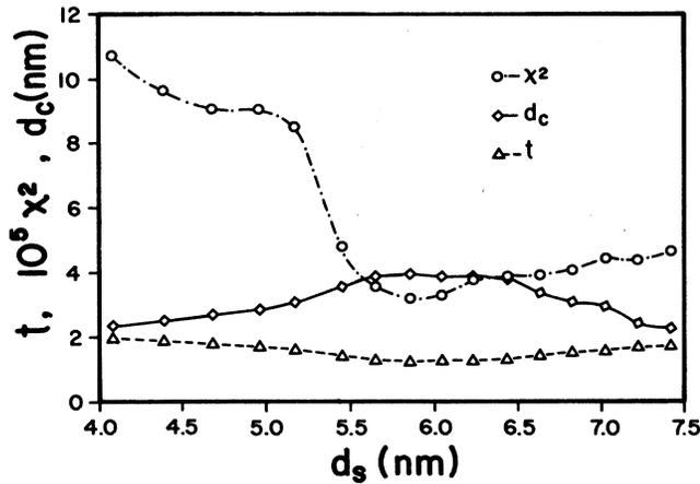
FIG. 3. The critical exponent  $t$ , the critical thickness  $d_c$ , and  $\chi^2$  vs the starting thickness  $d_s$ .
