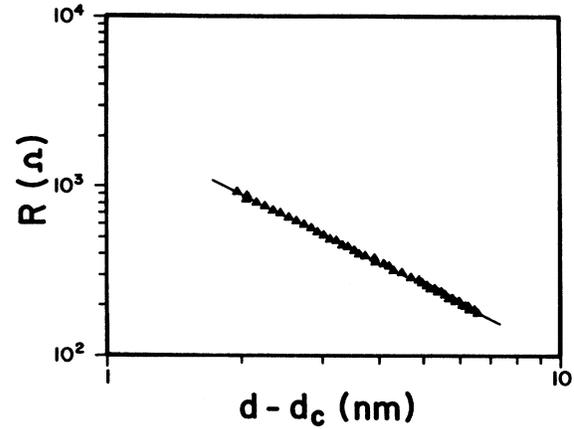
FIG. 5. The film resistance  $R$  vs  $(d - d_c)$  in the metal-insulator region. The slope of the straight line is 1.33 and the critical thickness is 3.84 nm.
