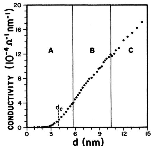
FIG. 2. Ni film conductivity vs thickness  $d$ . The critical thickness  $d_c$  is indicated by a dashed vertical line (not all data points are shown).
