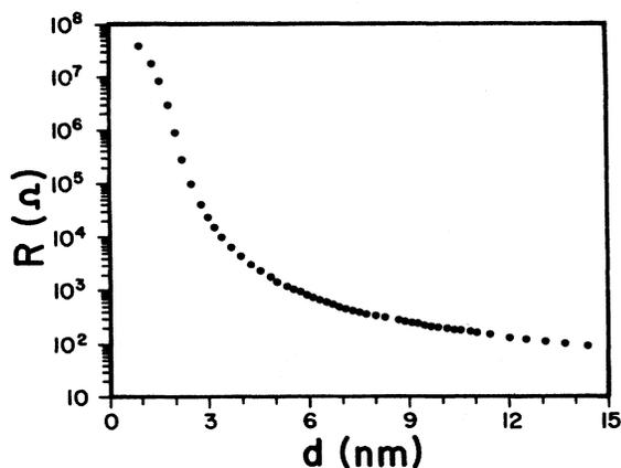
FIG. 1. The log of the resistance  $R$  vs thickness  $d$  for a Ni thin film.
