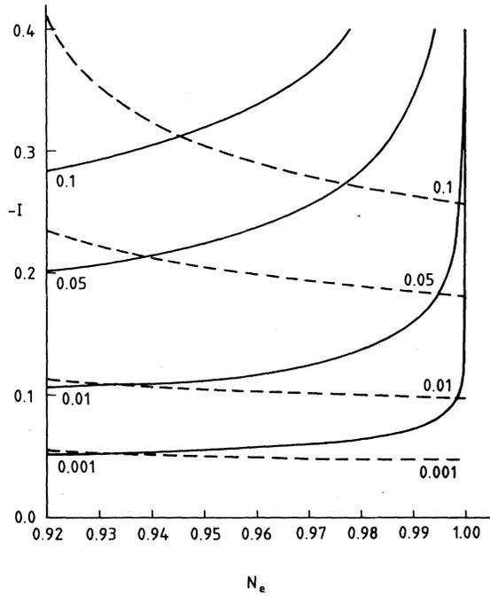
FIG. 1. Self-consistent solutions of the gap equations: Contours of constant  $\Delta$  (—) and constant  $g$  (---) as functions of the Hubbard  $I$  and the electron band filling  $N_e$ . The numbers to the right label the  $g$  contours, those to the left label the  $\Delta$  contours.
