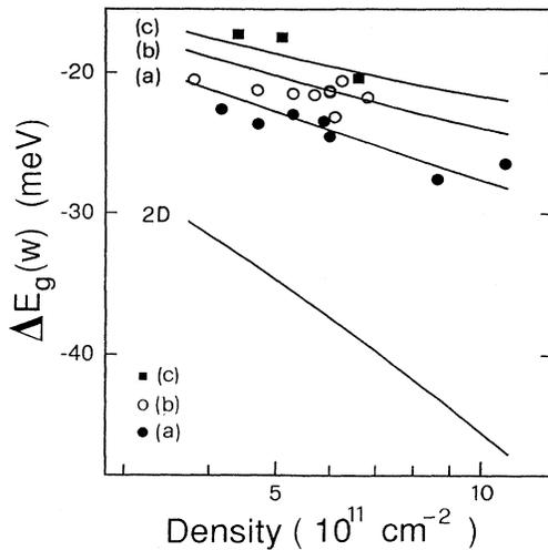
FIG. 3. Reduction of the band-gap width  $\Delta E_g(w)$  induced by an  $e-h$  plasma confined in a GaAs-(Ga,Al)As QW. The curves have been calculated in the SPPA using the “bulk” masses of Ref. 8 for a carrier temperature of 100 K; the labels on the left refer to the samples listed in Table I (2D refers to the two-dimensional case). The dots are experimental data obtained from a numerical analysis of the luminescence spectra as explained in the text.
