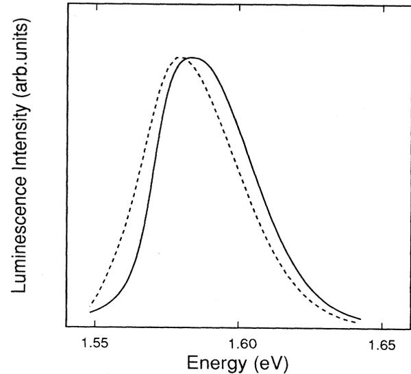
FIG. 4. Calculated luminescence spectra of an  $e-h$  plasma confined in a well of 80 Å width and having a density of  $7.5 \times 10^{11} \text{ cm}^{-2}$  and a temperature of 115 K. Dashed line, spectrum computed using Eq. (1); solid line, spectrum computed following Ref. 8 (see text).
