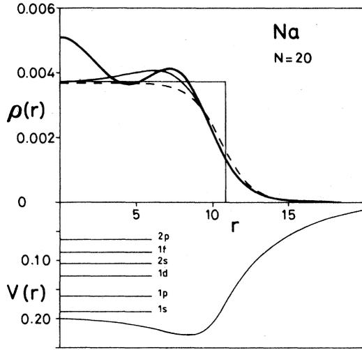
FIG. 1. Densities  $\rho(r)$  and single-electron potential  $V(r)$  (in a.u.) corresponding to the  $N=20$  Na cluster. The thick line is the KS density, whereas the thin one is the variational TF density. Also displayed are the adjusted TF density (dashed line) and the constant jellium density. The horizontal lines represent some of the single-electron levels. Starting from the bottom, they correspond to the 1s, 1p, 1d, 2s, 1f, and 2p states.
