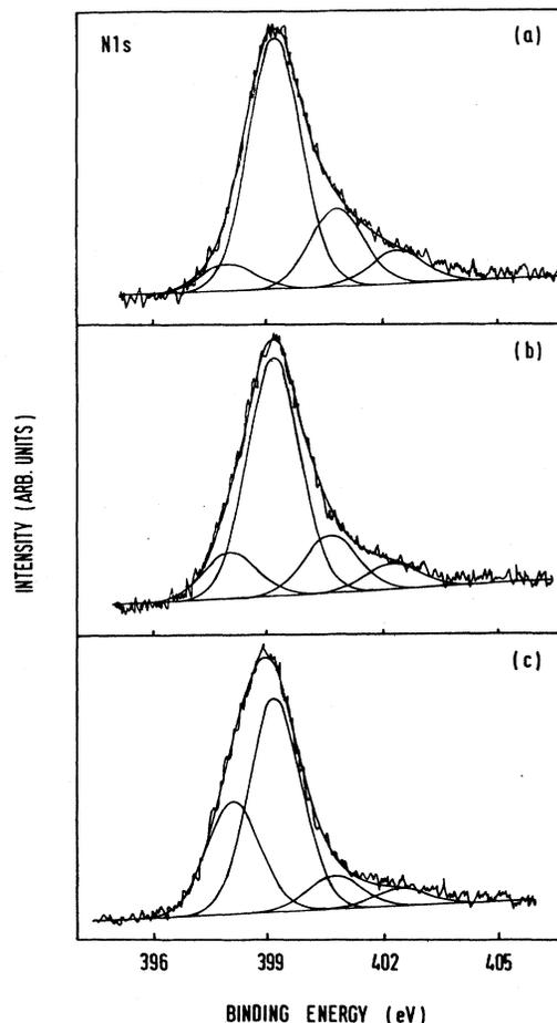
FIG. 2. N 1s XPS core-level spectra of polyemeraldine hydrochloride at various degree of protonation: (a) total [Cl]/[N]=0.44, (b) total [Cl]/[N]=0.28, and (c) total [Cl]/[N]=0.14.
