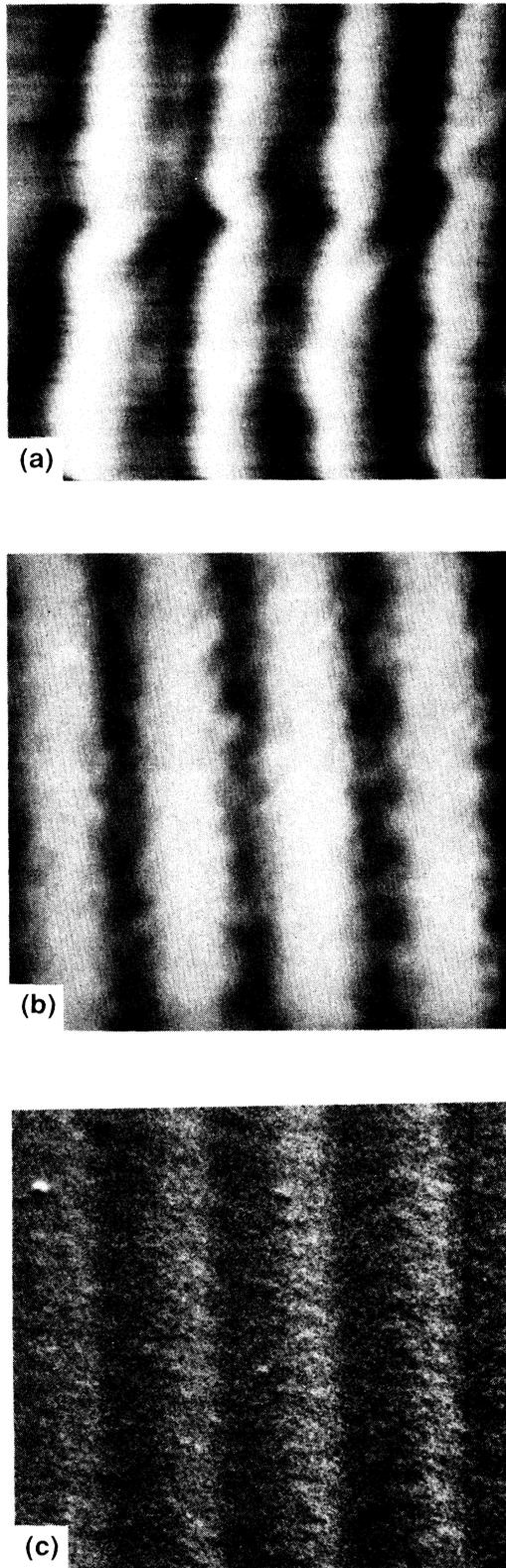
FIG. 3. Images of a holographic grating structure taken with (a) PSTM, (b) electron STM, and (c) scanning electron microscope. Actual line spacing is  $1.17 \mu\text{m}$ .
