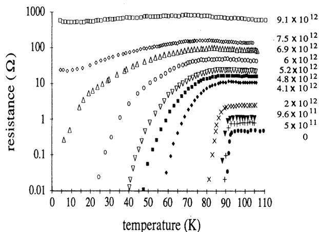
FIG. 1. *In situ* resistance measurements vs temperature for  $\text{YBa}_2\text{Cu}_3\text{O}_{6.9}$  bars irradiated at 105 K by 3.5-GeV xenon ions for different fluences.
