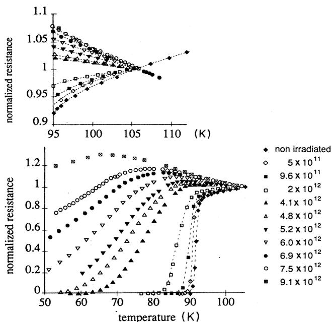
FIG. 2. Normalized transition curves of  $\text{YBa}_2\text{Cu}_3\text{O}_{6.9}$  irradiated by 3.5-GeV xenon ions. The upper figure is a magnification of the 100 K region. Note the continuous transition from metallic to semiconducting behavior.
