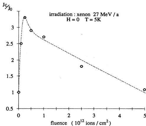
FIG. 6. Critical magnetization current density  $J_c/J_{c0}$  vs fluence at 5 K and zero field for  $\text{YBa}_2\text{Cu}_3\text{O}_{6.9}$  samples irradiated by 3.5-GeV xenon ions at 300 K. The dashed line is only a guide to the eye.
