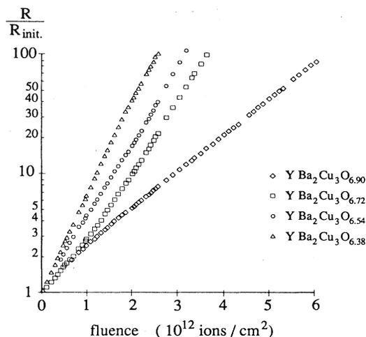
FIG. 4. Exponential variations of the resistance normalized to its initial value at 105 K for  $\text{YBa}_2\text{Cu}_3\text{O}_{7-\delta}$  oxides ( $\delta=0.10, 0.28, 0.46, 0.62$ ) irradiated by 3.5-GeV xenon ions.
