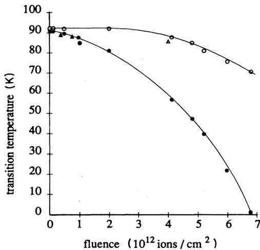
FIG. 8.  $T_c$  onset and  $T_c$  offset vs fluences for  $\text{YBa}_2\text{Cu}_3\text{O}_{6.9}$  samples irradiated at 105 K. The circles correspond to Xe irradiation ( $\odot$  is a room-temperature Xe irradiation), and the triangles to Kr irradiation.
