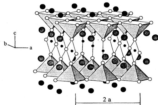
FIG. 9. Schematic drawing of the intergrowth of  $[\text{CuO}_2]_\infty$  and  $[\text{CuO}]_\infty$  chains appearing as local contrast modulations in  $\text{YBa}_2\text{Cu}_3\text{O}_{6.9}$  microcrystals irradiated by xenon ions at a dose of  $\phi t = 10^{12}$  cm<sup>-2</sup>.
