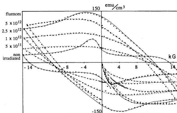
FIG. 5. Magnetic moment vs applied magnetic field at 5 K for  $\text{YBa}_2\text{Cu}_3\text{O}_{6.9}$  samples irradiated by 3.5-GeV xenon ions at 300 K for different fluences.
