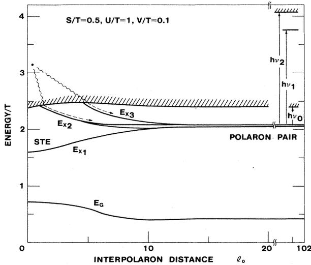
FIG. 3. Adiabatic energies as a function of  $l_0$ .  $\Delta Q$  and  $\theta$  are determined to minimize  $E_{x_1}$ .  $\Delta Q_- = 0$ .
