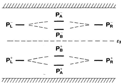
FIG. 4. Schematic nature of one-body energy levels that appeared within the gap. Upper (lower) shaded region corresponds to the electron (hole) continuum. Subscripts  $-$  and  $+$  of  $P$  correspond to the electron and the hole.  $L$  and  $R$  correspond to the left and the right when  $l_0 = \infty$ .  $B$  and  $A$  correspond to the bonding and antibonding states when  $l_0 \approx 6$ .
