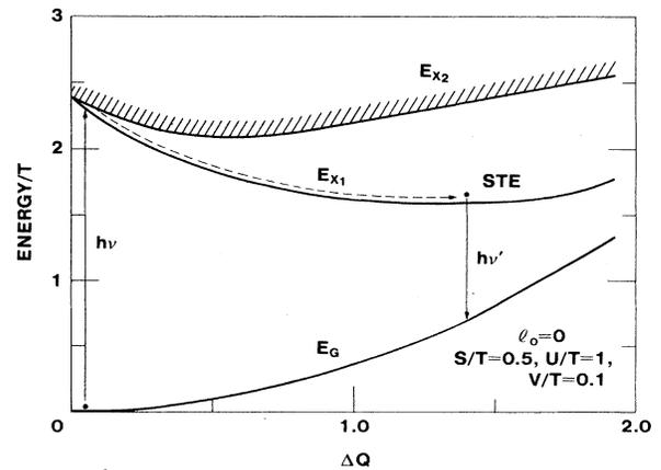
FIG. 2. Adiabatic energies as a function of  $\Delta Q$  at  $l_0 = 0$  and  $\Delta Q_- = 0$ .  $\theta$  is determined to minimize  $E_{x_1}$ .
