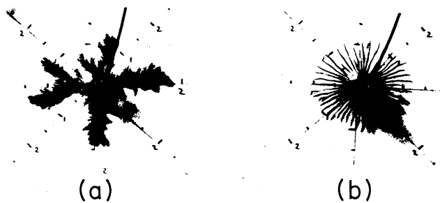
FIG. 2. Patterns associated with (a) incoherent and (b) coherent oscillations. (a) corresponds to n=0.5 M, V=5 V, after 800 sec of growth and (b) corresponds to n=0.05 M, V=10 V, after 300 sec of growth.
