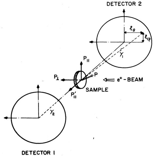
FIG. 2. The geometry of the 2D ACAR experiment:  $\theta = p_{\perp}/m_e c$ ,  $\phi = p_{\parallel}/m_e c$ , and  $p'_{\parallel}$  is integrated. The angle  $\theta$  and  $\phi$  are determined by the ratios of  $l_{\theta}$  and  $l_{\phi}$  to sample-to-detector distance.
