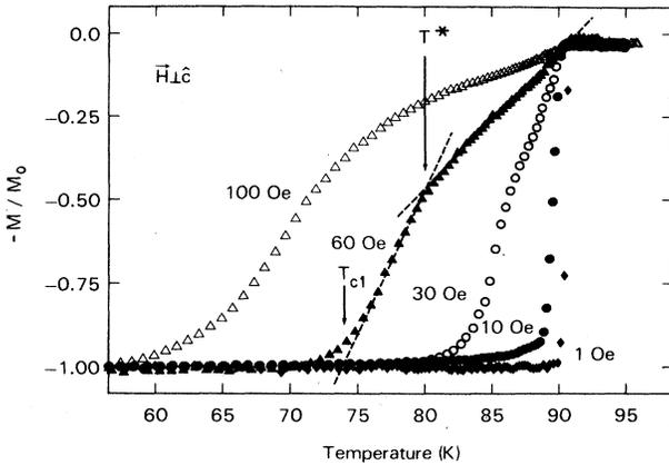
FIG. 1. Zero-field-cooled (ZFC) magnetization (normalized to its value at 4.2 K) of an Y-Ba-Cu-O crystal as a function of temperature, for several fields applied parallel to the  $a$ - $b$  plane. The temperature  $T_{c1}$ , at which the applied field equals  $H_{c1}/(1-N)$ , is identified from the linear extrapolation of the initial flux penetration as shown by the dashed lines.
