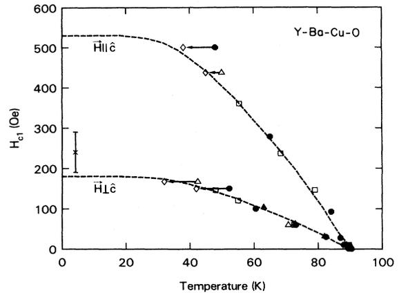
FIG. 3.  $H_{c1}$  for  $H$  applied parallel to the  $c$  axis and perpendicular to the  $c$  axis for several Y-Ba-Cu-O crystals. The  $T_{c1}$  corrections described in the text are indicated by the horizontal arrows. Low-temperature value for  $H_{c1}^\perp \hat{c} = 250 \pm 50$  Oe from Yeshurun *et al.* (Ref. 7) is shown as a cross (their value for  $H_{c1}^\parallel \hat{c}$  is  $900 \pm 100$  Oe). The dashed line represents to the clean-local-limit weak-coupling BCS prediction.
