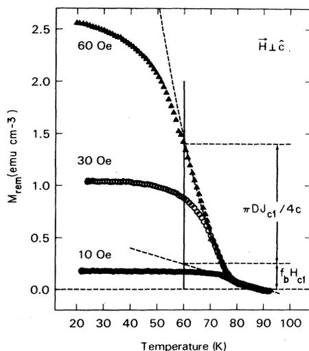
FIG. 2. Remanent magnetization of the same crystal as in Fig. 1, as a function of temperature for several fields applied parallel to the  $a$ - $b$  plane. The extrapolated line separates contributions to Eq. (3b) from  $H_{c1}$  and from  $J_c$ .
