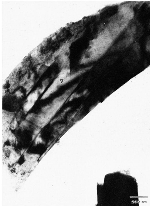
FIG. 6. Transmission electron microscopy (TEM) micrograph for a particle in sample 1. The arrow points to bend contour.
