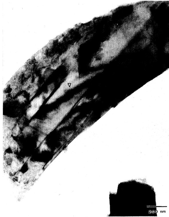
FIG. 6. Transmission electron microscopy (TEM) micrograph for a particle in sample 1. The arrow points to bend contour.
