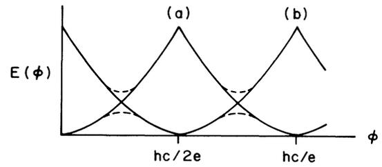
FIG. 4. Ground-state energy as a function of the electromagnetic flux through the cylinder in Fig. 3. Curve a is the branch corresponding to no statistical flux through the cylinder, curve b to half a flux quantum. The dashed curve includes the effect of mixing between the first two curves.
