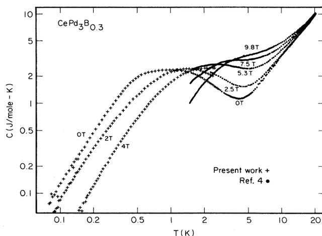
FIG. 3. The combined heat-capacity results of the present work and Ref. 4 shown on a  $\ln$ - $\ln$  plot. Not all of the experimental data points are shown for the sake of clarity.
