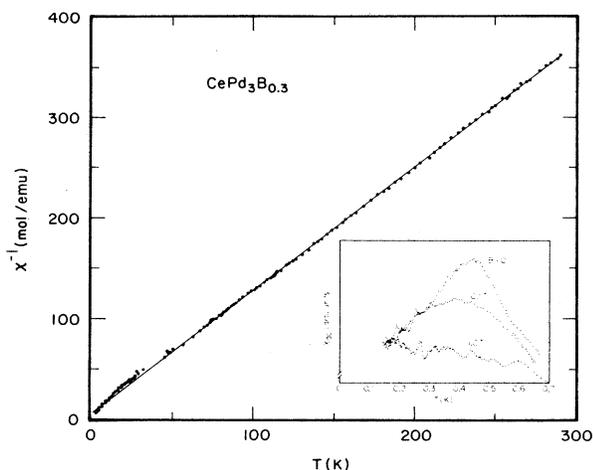
FIG. 1. The inverse molar susceptibility vs temperature of  $\text{CePd}_3\text{B}_{0.3}$  in an external field of 0.6 T. The inset shows ac susceptibility (117 Hz) from 0.15 to 0.7 K in zero and applied fields of 0.1 and 1 T.
