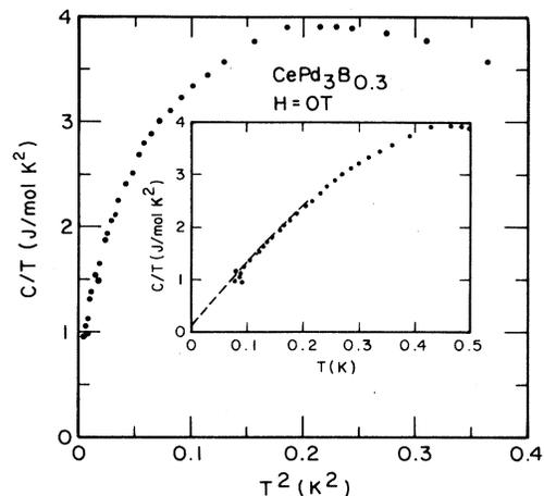
FIG. 4. The zero-field heat capacity of  $\text{CePd}_3\text{B}_{0.3}$  in the form of  $C/T$  vs  $T^2$  below 0.6 K. The inset shows  $C/T$  vs  $T$  and the dashed line is the linear extrapolation of the data below  $\sim 0.3$  K.
