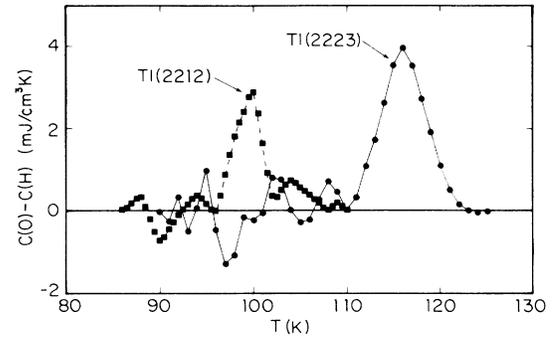
FIG. 5. Specific heat calculated from the curvature of the free-energy curves for both Tl (2:2:2:3) and Tl (2:2:1:2) at  $H=2$  T.
