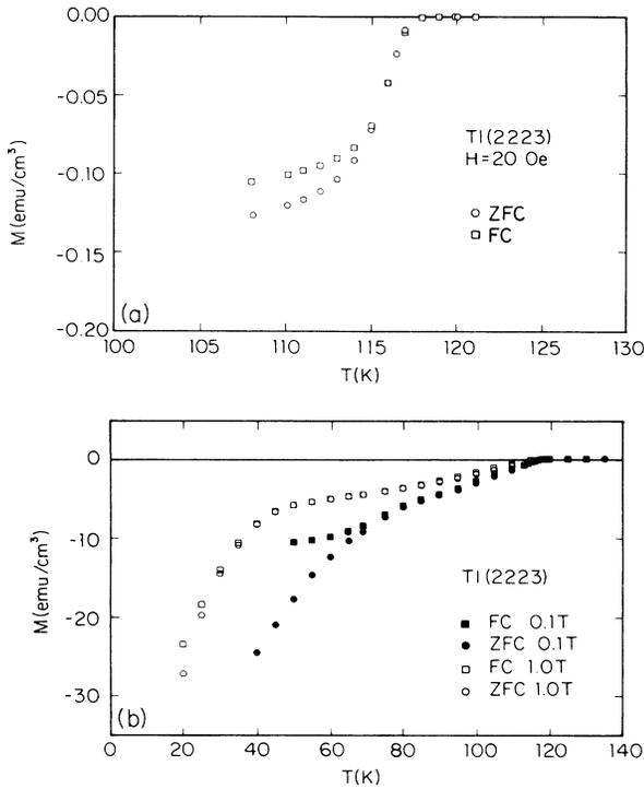
FIG. 1. (a) Temperature dependence of the magnetization for Tl (2:2:2:3) for low field of 20 Oe. (b) Temperature dependence of the magnetization for Tl (2:2:2:3) for 0.1 and 1.0 T.
