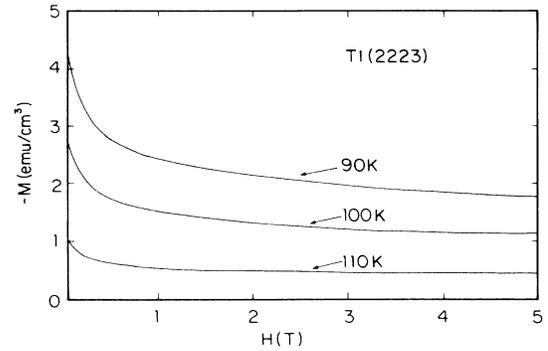
FIG. 3. Magnetization ( $M$ -vs- $H$ ) curves for Tl (2:2:2:3).
