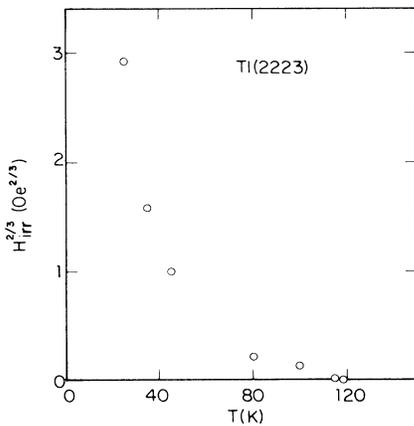
FIG. 2. Thermodynamic irreversibility for the Tl (2:2:2:3) curve defined as the temperature and field point where the magnetization changes by less than 1% in 20 min.
