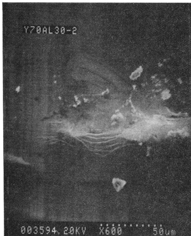
FIG. 1. (a) Sample of Y_{70}Al_{30} showing damaged area due to the spot-welding of a 0.09-mm-diam copper wire; (b) enlargement of the same area.
