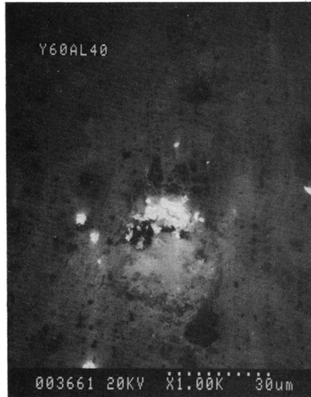
FIG. 2. (a) Detail of the area between the two Hall contacts made by bonding ultrasonically very small aluminum wires; (b) enlargement of the similar contact area with the aluminum wire removed.
