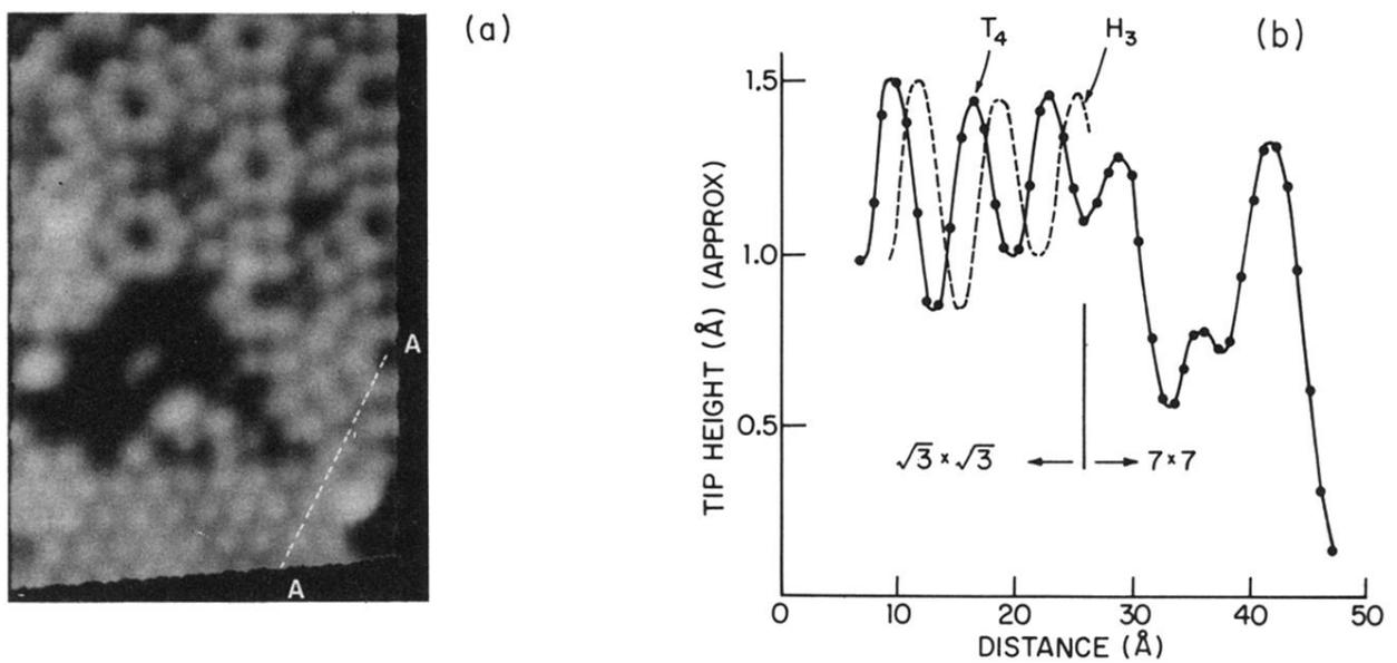
FIG. 1. (a) Tunneling imaging showing  $(7 \times 7)$  and  $(\sqrt{3} \times \sqrt{3})R 30^\circ$  reconstructions on a partially gallium covered silicon (111) surface for tip bias of  $-1.1$  V and tunnel current of 1 nA. (b) Line scan of top height along the  $A$ - $A$  section shown in Fig. 1. The dotted line shows how scan would look for  $H_3$ -type reconstruction. Heights of atoms in  $(\sqrt{3} \times \sqrt{3})$  are similar to  $(7 \times 7)$ , confirming the adatom model.
