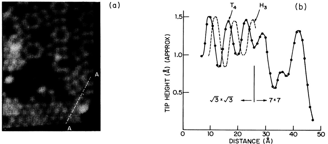
FIG. 1. (a) Tunneling imaging showing  $(7 \times 7)$  and  $(\sqrt{3} \times \sqrt{3})R30^\circ$  reconstructions on a partially gallium covered silicon (111) surface for tip bias of  $-1.1$  V and tunnel current of 1 nA. (b) Line scan of top height along the  $A-A$  section shown in Fig. 1. The dotted line shows how scan would look for  $H_3$ -type reconstruction. Heights of atoms in  $(\sqrt{3} \times \sqrt{3})$  are similar to  $(7 \times 7)$ , confirming the adatom model.
