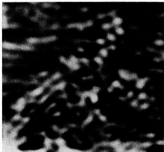
FIG. 2. 40 \times 40 \text{ \AA}^2 STM image of a -C film taken in the barrier-height mode (crystal bias +20 mV).
