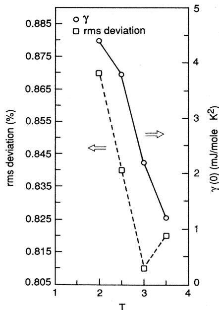
FIG. 4. The coefficient of the linear term derived from a fit of the Tl-Ca-Ba-Cu-O single-crystal data to Eq. (1), and the rms deviation of the data from the fit, are plotted against the lowest temperature included in the fit. All fits include data up to 11 K. The linear term tends to zero when the data below 3.5 K, which cannot be accurately modeled, are excluded.
