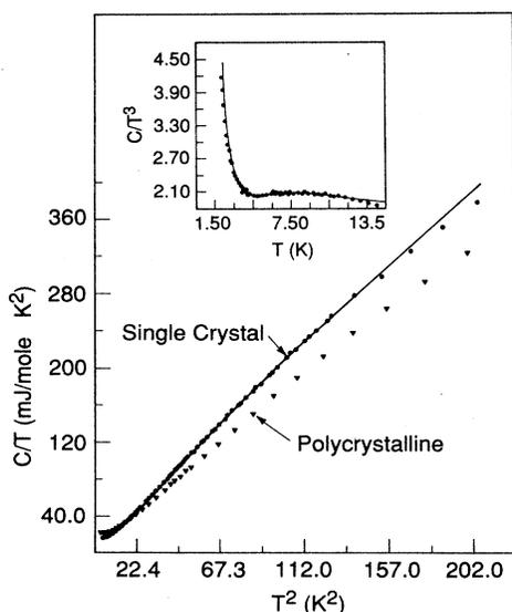
FIG. 3.  $C/T$  vs  $T^2$  for the Tl-Ca-Ba-Cu-O single crystal and polycrystalline samples. The line represents the best fit of the single crystal to Eq. (1) in the range 3.5–11 K, showing a linear term of 1 mJ/mole  $K^2$ . Inset:  $C/T^3$  vs  $T$  for the single crystal with the same fit.
