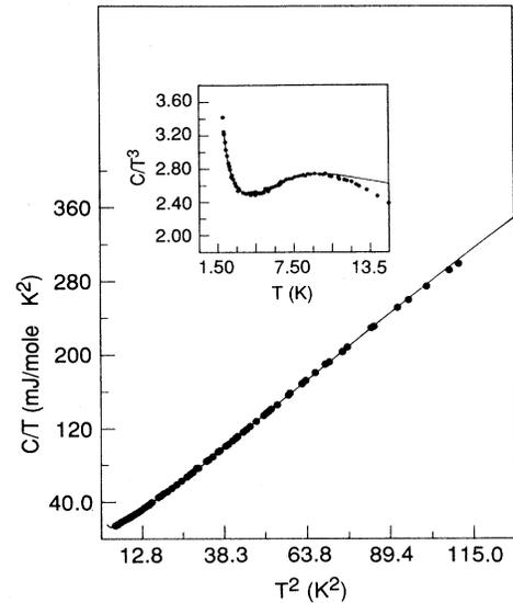
FIG. 2.  $C/T$  vs  $T^2$  for Bi-Ca-Sr-Cu-O single crystal. The line represents the best fit to Eq. (1) in the range 2–11 K showing a linear term of  $0.6$  mJ/mole  $K^2$ . Inset:  $C/T^3$  vs  $T$  with the same fit.
