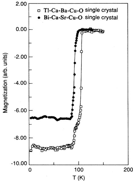
FIG. 1. Magnetization of Tl-Ca-Ba-Cu-O and Bi-Ca-Sr-Cu-O single crystals cooled in  $\approx 1$  G.
