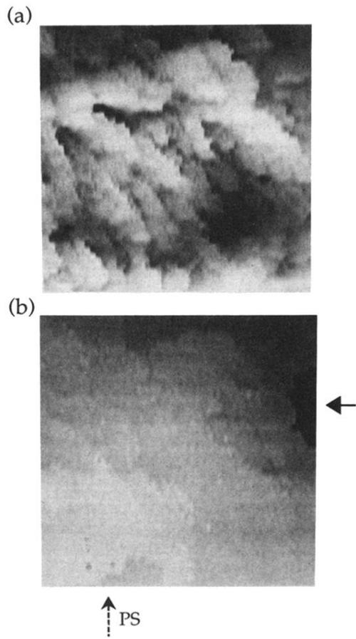
FIG. 3. (a) Topographic and (b) potentiometric gray scale images of a Y-Ba-Cu-O thin film acquired simultaneously with an applied field of 8 V/cm (applied from left to right in these figures). The images are of a  $5\ \mu\text{m} \times 5\ \mu\text{m}$  area. For topography the gray scale is 2000 Å from black (low) to white (high) and for potentiometry the scale is 15 mV from black (low potential) to white (high potential).
