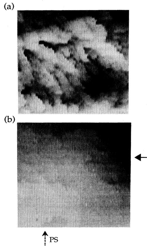
FIG. 3. (a) Topographic and (b) potentiometric gray scale images of a Y-Ba-Cu-O thin film acquired simultaneously with an applied field of 8 V/cm (applied from left to right in these figures). The images are of a  $5 \mu\text{m} \times 5 \mu\text{m}$  area. For topography the gray scale is 2000 Å from black (low) to white (high) and for potentiometry the scale is 15 mV from black (low potential) to white (high potential).
