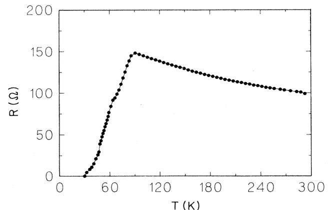
FIG. 1. Resistive superconducting transition of a disordered polycrystalline Y-Ba-Cu-O thin film (resistance per square vs temperature).
