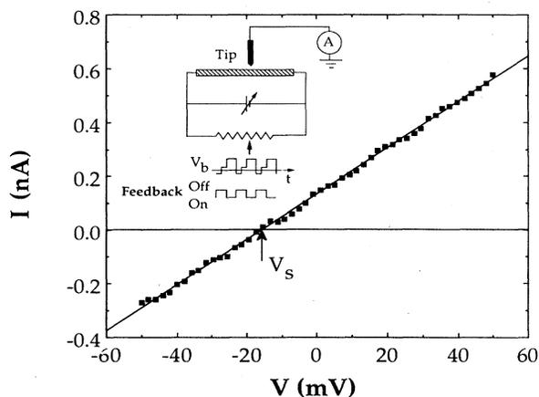
FIG. 2. Typical  $I$ - $V_b$  curve showing the linear current-voltage characteristics and the determination of the sample potential from this measurement. The inset of this figure shows the circuit and waveforms used for scanning tunneling potentiometry.
