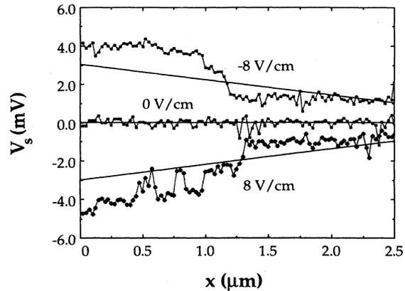
FIG. 4. Single line scans across the step indicated with a solid arrow in Fig. 3(b) along the direction of the applied field  $x$ . The curves from top to bottom are applied fields of  $-8$ ,  $0$ ,  $8 \text{ V/cm}$  respectively. The top and bottom curves have been offset from zero for clarity. The uniform potential distribution expected for these applied fields are also shown (solid straight lines).
