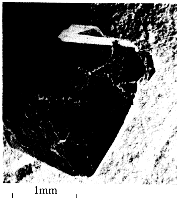
FIG. 7. SEM picture of a RuS 2 single crystal after 20 h of photochemical oxidation by white light in 1N H 2 SO 4 at 1.0 V with respect to the saturated calomel electrode.
