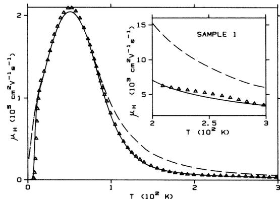
FIG. 1. Hall mobility of sample 1. The solid line is the fit of the full model to the data. The dashed line is obtained when the deep centers are not accounted for and the dash-dotted line corresponds to the absence of impurity conduction.
