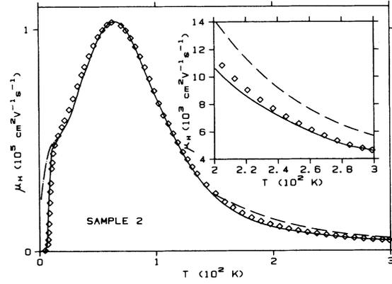
FIG. 3. Hall mobility of sample 2. The lines are as for Fig. 1.
