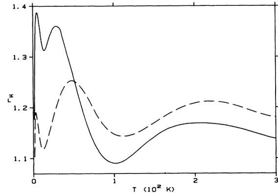
FIG. 5. Hall factor as a function of temperature. The solid line corresponds to sample 1 and the dashed one to sample 2.
