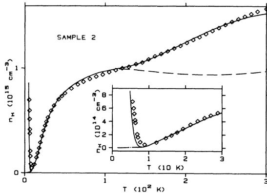
FIG. 4. Hall electronic concentration for sample 2. The lines are as for Fig. 1.
