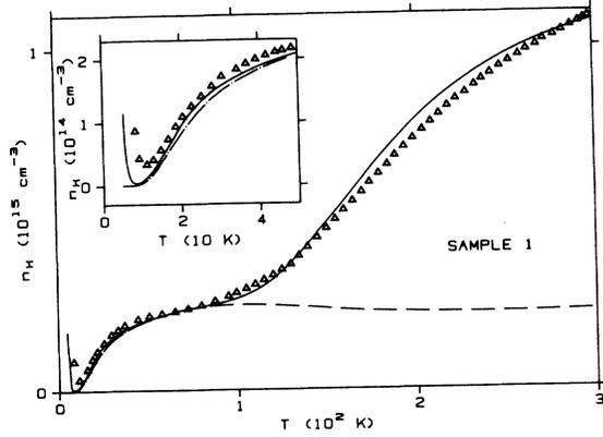
FIG. 2. Hall electronic concentration for sample 1. The lines are as for Fig. 1.
