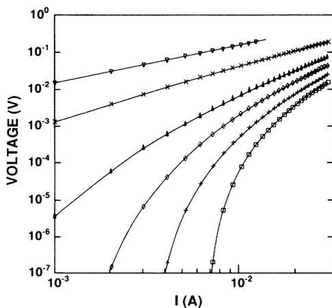
FIG. 2. The current voltage characteristics of the high-temperature superconducting film recorded at a sequence of temperatures. From the bottom: 11, 30, 40, 50, 60, and 80 K.
