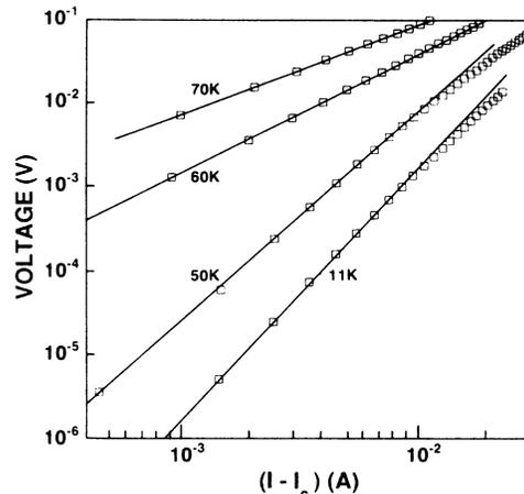
FIG. 3. The current voltage characteristics of the film both below (11 K, 50 K) and above (60 K, 70 K) the coherence transition.
