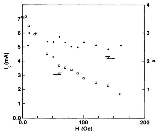
FIG. 5. The behavior of the critical current (squares) and the parameter  $x$  (filled circles), as a function of the perpendicular field intensity  $H$  at  $T = 4.2$  K.
