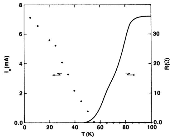
FIG. 1. The resistive transition of the high-temperature superconducting film measured at  $0.7 \text{ A/cm}^2$  (solid line) and the critical current evaluated using a  $1\text{-}\mu\text{V/mm}$  criterion (filled circles). The critical current density at 4.2 K is  $\sim 700 \text{ A/cm}^2$ .
