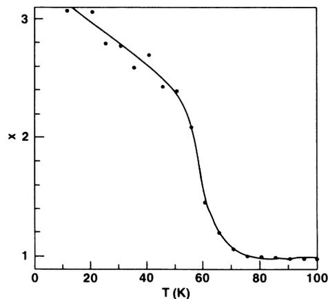
FIG. 4. Behavior of the critical parameter  $x$  which appears in  $V \sim (I - I_c)^x$  as a function of temperature. The sharp rise from  $\sim 1$  to  $\sim 2$  at  $T_c \sim 60$  K is interpreted as the coherence transition.
