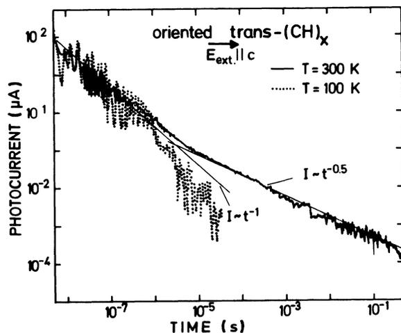
FIG. 5. Decay of the photocurrent after 500-ps excitation investigated from nanoseconds to seconds at 300 K (solid line) and at 100 K (dotted line).
