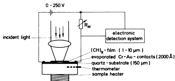
FIG. 1. Schematic setup for measuring the photocurrent. The resistance  $R_M$  is in most cases the input resistance of the electronic detection system.
