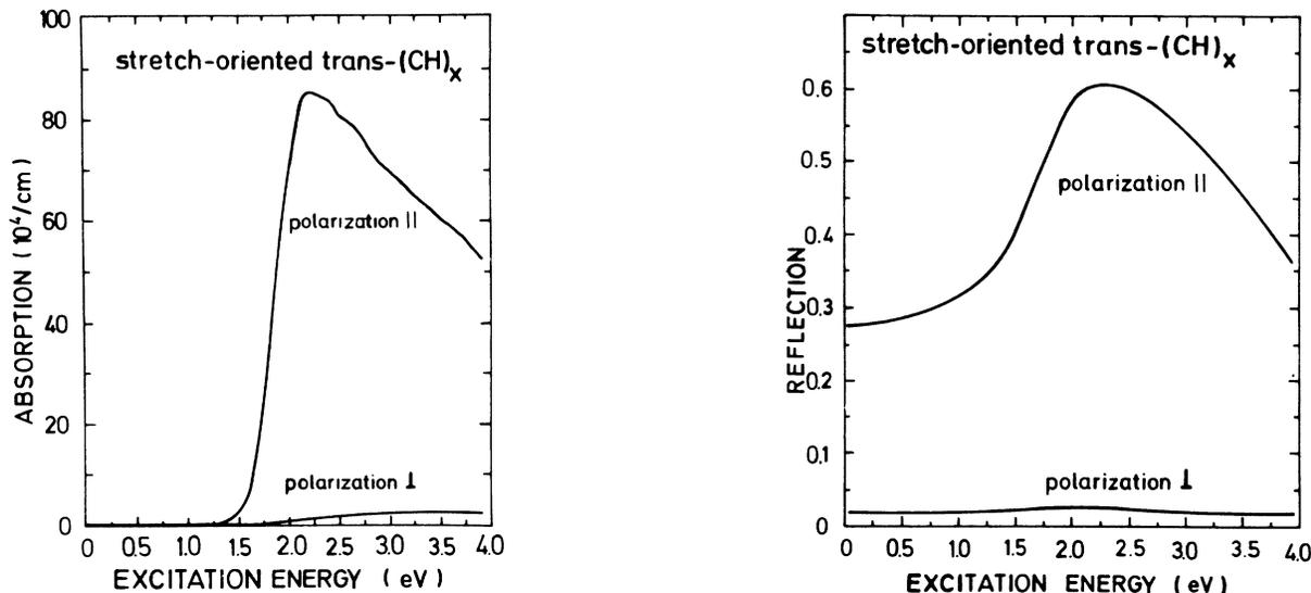
FIG. 10. Absorption and reflection spectra of highly oriented Durham-Graz-type polyacetylene obtained from Refs. 31 and 32.
