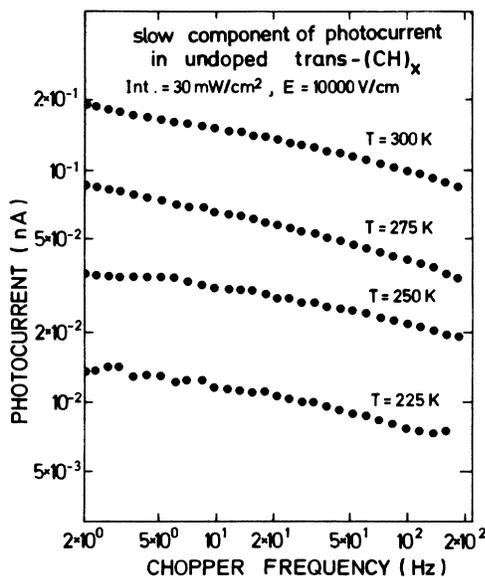
FIG. 6. The slow-PC component as function of the chopper frequency at four different temperatures on a log-log plot.
