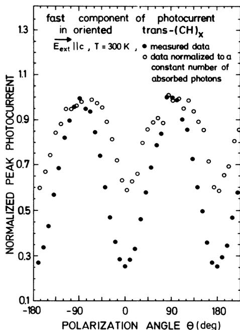
FIG. 11. Anisotropy of the fast-PC component with respect to the polarization of the incident light.  $\theta$  is the angle between the polarization and the chain direction. Excitation energy is 2.6 eV.
