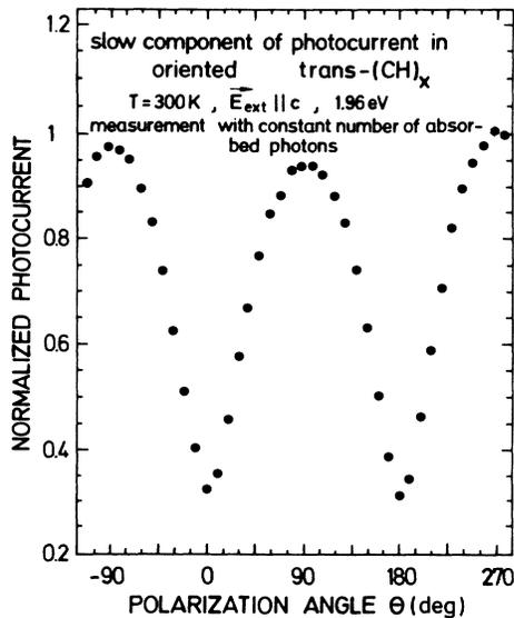
FIG. 12. Polarization anisotropy of the slow-PC component excitation energy is 2.1 eV. In this case the signal amplitudes have been measured directly at a constant number of absorbed photons by changing the intensity of the incident light in a sufficient way (instead of a numerical correction after the measurement as done in Fig. 11).
