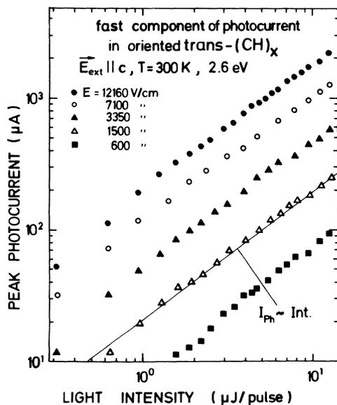
FIG. 3. Intensity dependence of the fast-PC component on a log-log plot at different electric fields. The slope of 1.0 clearly demonstrates the linear behavior between the peak photocurrent and the light intensity.
