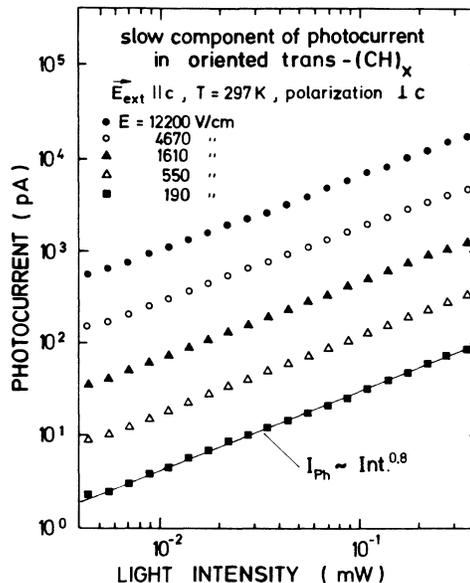
FIG. 9. Intensity dependence of the slow-PC component on a log-log plot. In the case of a polarization perpendicular to the chain direction (in oriented samples) the photocurrent goes with  $(\text{intensity})^{0.8}$ ; in other cases [parallel polarization or Shirakawa-type  $(\text{CH})_x$ ] the exponent has a value of 0.6–0.7.
