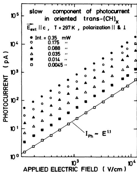
FIG. 8. Field dependence of the slow-PC component on a log-log plot at different light intensities. The photocurrent is proportional to  $E^{1.1}$  similar to the behavior of the fast component.
