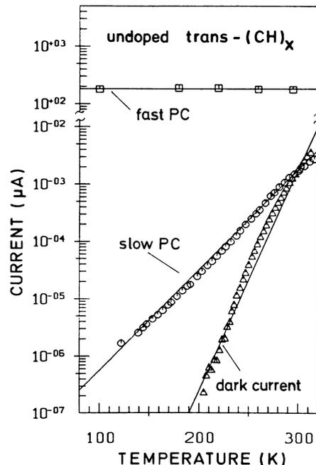
FIG. 7. Temperature dependence of the fast- and slow-PC component and of the dark current. The fast component is temperature independent down to about 10 K. The room-temperature value of the dark conductivity is  $7 \times 10^{-7}$  S/cm.
