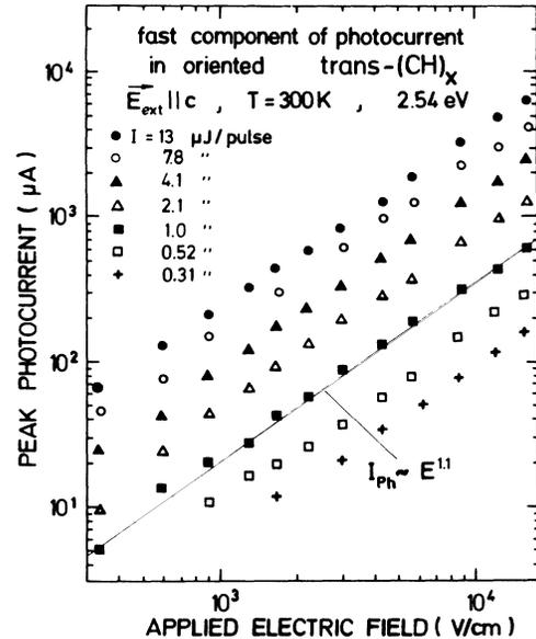
FIG. 4. Field dependence of the fast-PC component on a log-log plot at different intensities. The peak photocurrent  $I_{\text{ph}}$  is proportional to  $E^{1.1}$ .
