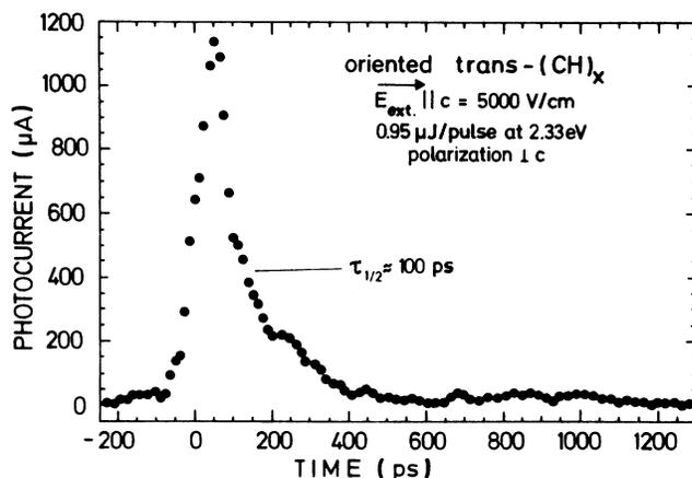
FIG. 2. Fast component of the photocurrent in  $\text{trans}-(\text{CH})_x$  excited with 25-ps laser pulses;  $T = 300$  K. The energy of the incident light pulses is 0.95  $\mu\text{J}$  at a sample area of  $200 \mu\text{m} \times 330 \mu\text{m}$ . The integral under the peak corresponds to  $1.5 \times 10^6$  electronic charges.
