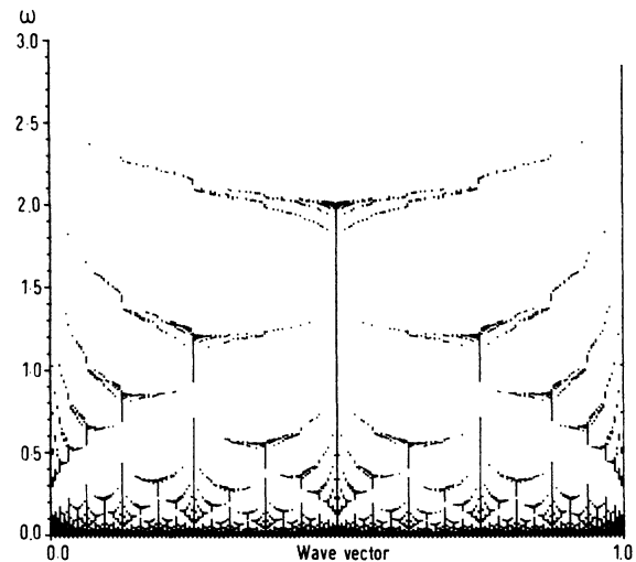
FIG. 4. Spectra of the modulated spring model with \Delta=1 for a selection of commensurate modulation wave vectors (Ref. 23). These are chosen as consecutive Farey numbers Q(n, j) , where n=1, 2, 3, \dots, 7 and j=1, \dots, 2^n . These are defined as follows. Q(1, 1)=0/1 , Q(1, 2)=1/1 . A Farey number at level m is obtained from two consecutive ones p/q and p'/q' at level m-1 as (p+p')/(q+q') .
