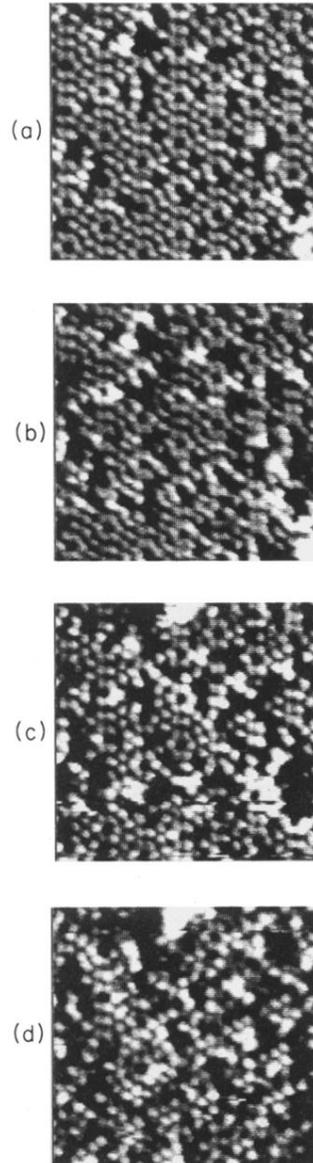
FIG. 1. STM pseudo-grey-scale images of oxygen on Si(111)-(7 $\times$ 7) for (a) 0-, (b) 2.4-, (c) 4.0-, and (d) 8.6-L exposure. Protrusions and depressions on the surface are represented by bright and dark regions, respectively.
