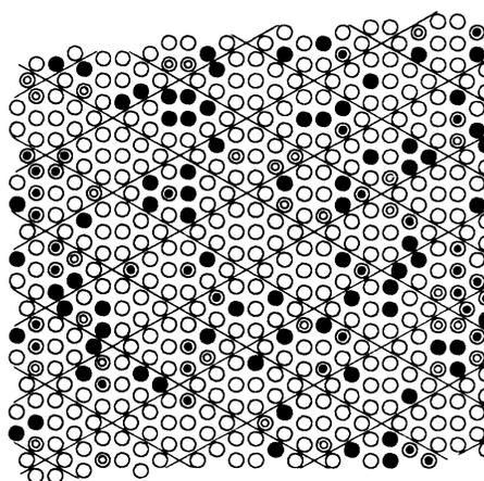
FIG. 2. Schematic diagram representing the images shown in Fig. 1. The lines indicate the surface (7×7) unit cells. The adatom sites are shown as circles. The “missing-adatom defects” in the image of Fig. 1(a) are indicated by filled circles. Newly generated “missing adatoms” in Figs. 1(b) and 1(c) are indicated by circles with a smaller filled circle at the center and circles with a smaller open circle at the center, respectively.
