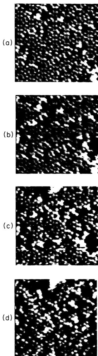
FIG. 1. STM pseudo-grey-scale images of oxygen on Si(111)-(7×7) for (a) 0-, (b) 2.4-, (c) 4.0-, and (d) 8.6-L exposure. Protrusions and depressions on the surface are represented by bright and dark regions, respectively.
