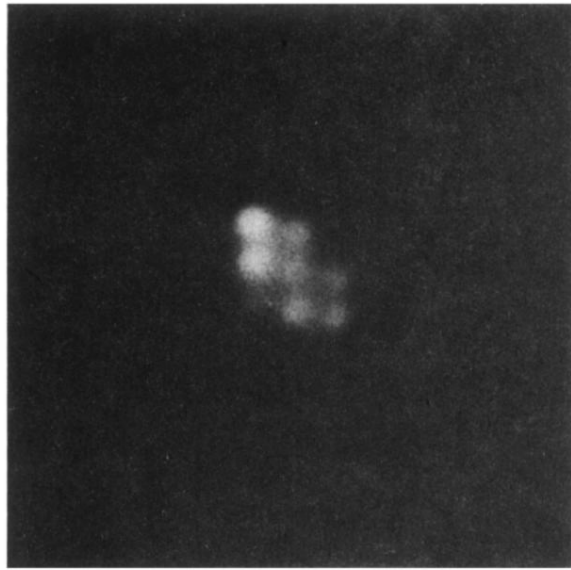
FIG. 4. Helium-neon field-ion micrograph of eight Pd atoms on the Ta(110) plane which comprised part of the interior of a two-dimensional cluster of \sim 30 atoms; imaged by the partial field evaporation of the original large cluster.
