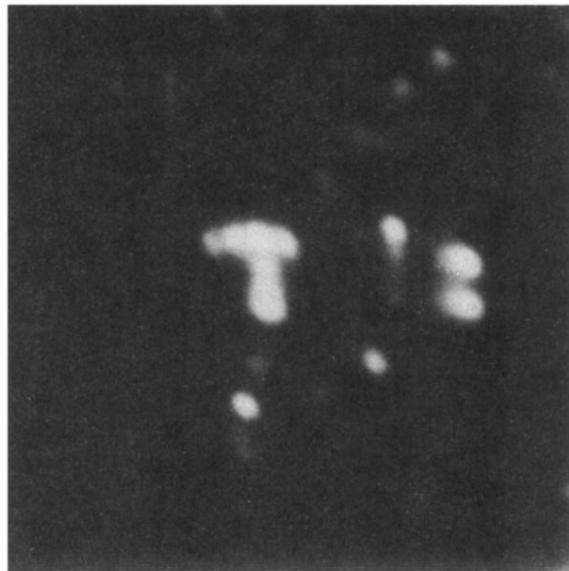
FIG. 7. Helium-neon field-ion micrograph of a configuration assumed by seven Pd atoms on a Ta(110) plane having a diameter sufficient to accommodate only about six Pd atoms in a single chain in a \langle 111 \rangle direction.
