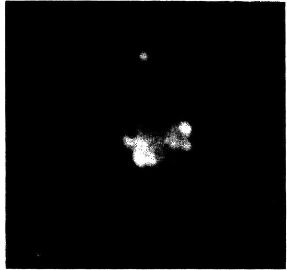
FIG. 3. Helium-neon field-ion micrograph of a two-dimensional cluster of 16 Pd atoms on Ta(110).
