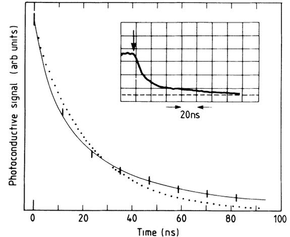
FIG. 1. Photoconductive signal after termination of the laser pulse ( $t=0$ ) for sample 1 at temperature ( $T$ ) of 4.2 K and bias electric field 1.2 V/cm. Dotted line, best exponential fit; solid line, see text. Inset shows the actual signal;  $t=0$  is indicated with an arrow.
