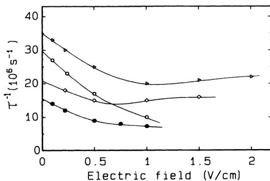
FIG. 4.  $\tau^{-1}$  as a function of bias electric field for several samples at full laser power at  $T=4.2 \text{ K}$ . A linear dependence for the data at the lowest bias fields is indicated.  $\nabla$ , sample 1;  $\circ$ , sample 2;  $\diamond$ , sample 6;  $\bullet$ , sample 4.
