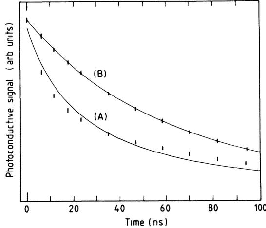
FIG. 8. Normalized photoconductive signal after  $t=0$  for sample 3 at  $T=3$  K, and bias electric field of 1.0 V/cm. Fits to data at (A) 100% and (B) 7.5% laser intensity.
