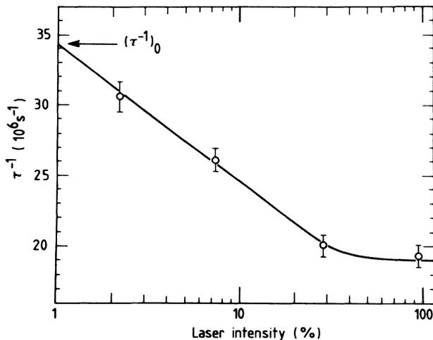
FIG. 6.  $\tau^{-1}$  obtained from a series of fits of the photoconductive decay for sample 1 as a function of incident FIR intensity at  $T=2$  K and a bias electric field of 1.0 V/cm. The line is meant to guide the eye.
