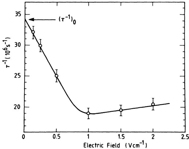
FIG. 3.  $\tau^{-1}$  obtained from a series of fits of the photoconductive decay for sample 1 as a function of bias electric field at full laser power at  $T=2 \text{ K}$ . A linear dependence for the data at the lowest bias fields is indicated.
