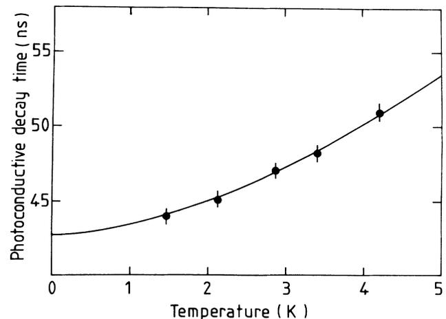
FIG. 2. Temperature dependence of the photoconductive decay time for sample 1 at a bias electric field of  $0.8 \text{ V cm}^{-1}$ . The solid line is a simple power-law fit to the data points and corresponds to an exponent of  $1.7 \pm 0.1$ .
