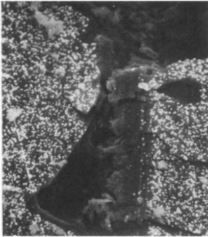
FIG. 14. Overview of a formation process of diamond film: (a) after 3 h, (b) after 12 h, and (c) after 30 h. The substrate is Si polished with a diamond paste. The dark area in the center is a scratch mark given on the substrate before the synthesis, and it is seen that the nucleation density of diamond particles is very low on the fresh Si surface.
