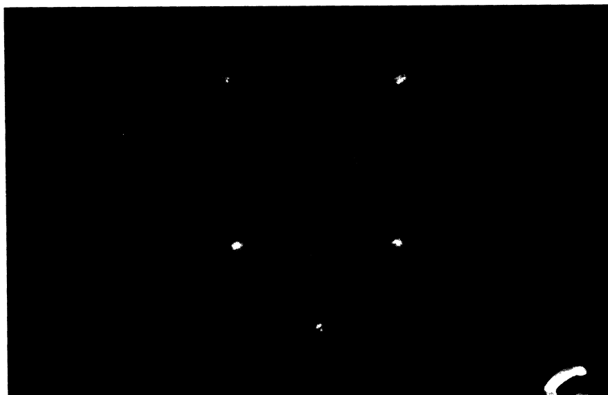
FIG. 13. LEED pattern of a krypton monolayer adsorbed on MgO(100) at T = 41.8 K and P = 1.2 \times 10^{-8} torr. Electron energy is 115.7 eV. As for Fig. 7, the most intense spots are from MgO. The Kr overlayer gives a weak ring, on which are superimposed four sets of doublets. The ring is probably due to a hexagonal packing of Kr atoms with crystallites orientationally disordered coexisting with a 2 \times n ( n \approx 8 ) structure (doublets).
