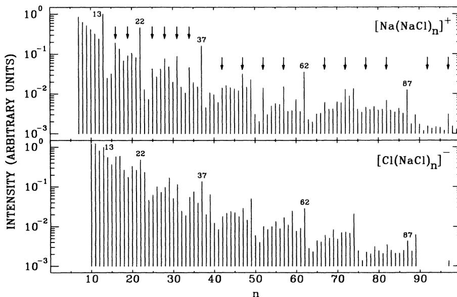
FIG. 2. Relative abundances of the positive and negative NaCl cluster ions, obtained by integrating the total charge detected at each mass. Cuboid cluster sizes at  $n = 13, 22, 37, 62,$  and  $87$  are clearly visible, along with a periodic fine structure. Single-mass population uncertainty is  $\pm 10\%$ . For distant comparisons, there is an additional uncertainty of  $\pm 2\%$  to the power  $\Delta n$ .
