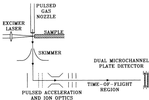
FIG. 1. Experimental apparatus: Cluster ions are produced by laser photofragmentation of the sample, cooled and entrained in the gas jet, and dispersed according to mass following acceleration to 10 keV.
