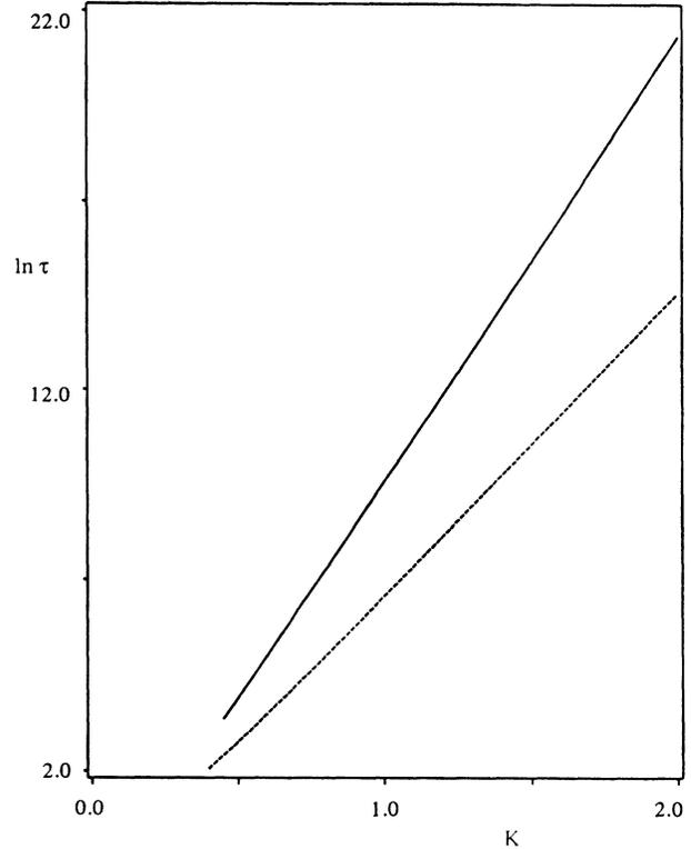
FIG. 2. A plot of  $\ln \tau$  against  $K$  for the 6 site (dotted curve) and 15 site (solid curve) Sierpiński gasket.
