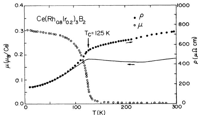
FIG. 1. Electrical resistivity  $\rho(T)$  and magnetic moment per Ce ion  $\mu(T)$  (in an applied field of 1 T) of pseudoternary compound  $\text{Ce}(\text{Rh}_{0.8}\text{Ir}_{0.2})_3\text{B}_2$  with Curie temperature  $T_C=125$  K. The local minimum of resistivity at 210 K can be easily seen in the cool-down curve.
