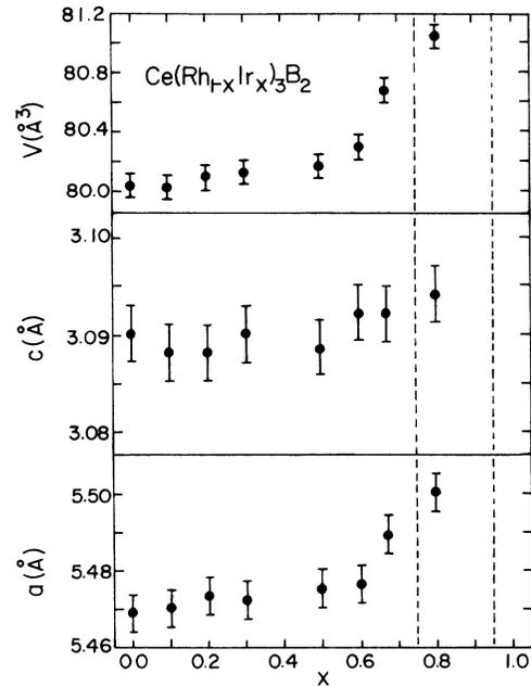
FIG. 4. Hexagonal lattice parameters ( $a$  and  $c$ ) and unit-cell volume  $V$  in the  $\text{Ce}(\text{Rh}_{1-x}\text{Ir}_x)_3\text{B}_2$  system. A two-phase region appears between  $x=0.75$  and  $x=0.95$ .
