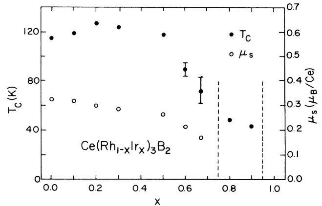
FIG. 3. Composition variation of Curie temperature  $T_C$  and saturation magnetic moment per Ce ion of the pseudoternary system  $\text{Ce}(\text{Rh}_{1-x}\text{Ir}_x)_3\text{B}_2$ . A two-phase region appears between  $x = 0.75$  and  $x = 0.95$ .
