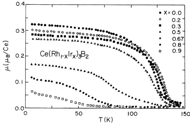
FIG. 2. Temperature dependence of magnetization (in magnetic moment per Ce ion) of  $\text{Ce}(\text{Rh}_{1-x}\text{Ir}_x)_3\text{B}_2$  powder samples in an applied field of 1 T.
