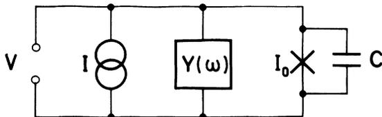
FIG. 1. Equivalent circuit of a current-biased Josephson junction.
