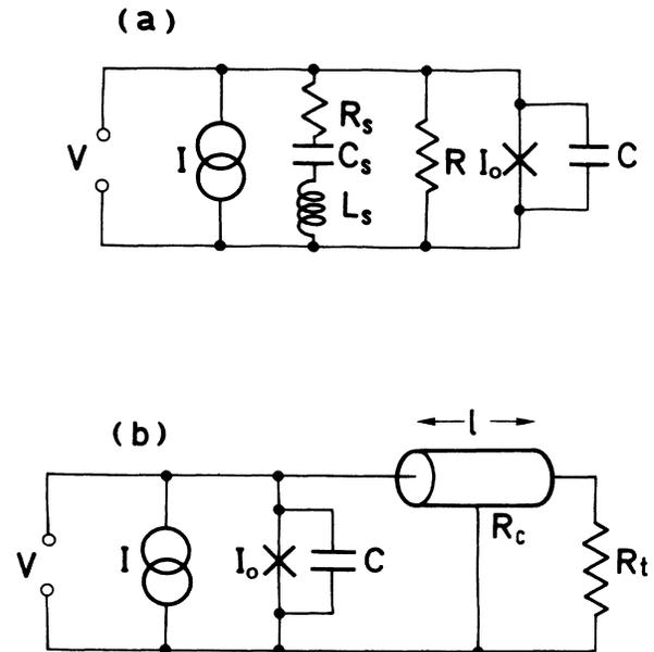
FIG. 4. Junction circuit models for two cases of non-Ohmic dissipation. (a) Admittance loading consisting of a resistor in parallel with  $RLC$  resonant circuit. (b) Admittance arising from a transmission line of characteristic impedance  $R_c$ , length  $l$ , and terminated by resistor  $R_t$ .
