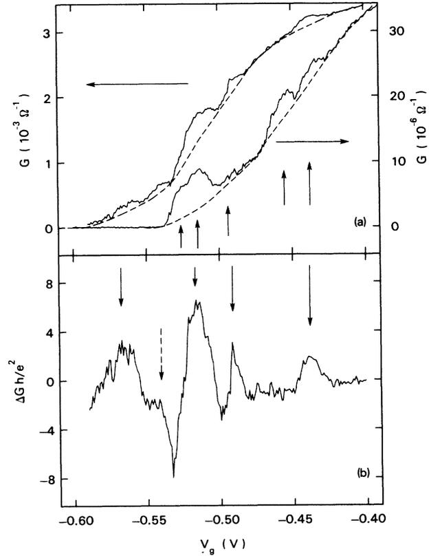
FIG. 2. The dependence of the conductance  $G(V_g)$  on gate voltage near threshold at 0.02 K for sample 1 (left axis) and sample 2 (right axis). The arrows mark the positions of the peaks in the conductance of sample 2. The dashed lines are *ad hoc* estimates of the classical  $G(V_g)$  described in the text. (b) The fluctuations in the  $G(V_g)$  from sample 1. The arrows mark the positions of the peaks in  $G(V_g)$ .
