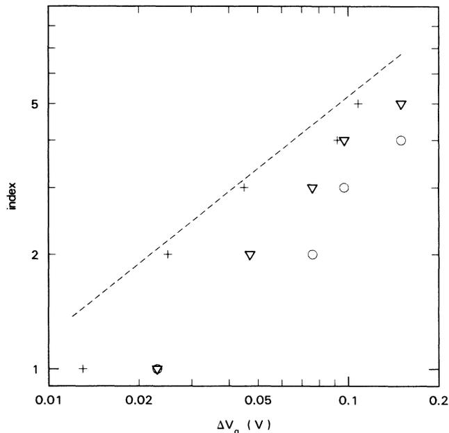
FIG. 3. Relative positions  $V_{\text{peak}} - V_T$  of the peaks (○) in  $\Delta G$  as a function of  $V_g$ , and positions of the peaks from sample 1 (▽) and sample 2 (+) derived by assuming that  $\Delta G$  is never less than zero. The dashed line illustrates the slope of the prediction for the resonances from a square barrier.
