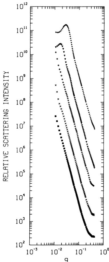
FIG. 2. Small-angle x-ray scattering curves for Electronu- cleonics, Inc. controlled-pore glasses with measured average pore sizes (from top to bottom): 86, 167, 477, 810, and 2023 Å. The values of  $q$  are given in  $\text{\AA}^{-1}$ .
