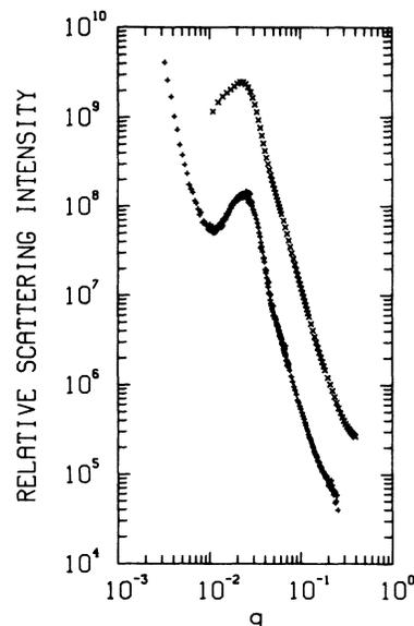
FIG. 1. The relative small-angle x-ray scattering (upper curve) and small-angle neutron scattering (lower curve) from Vycor<sup>®</sup> controlled-pore glass. On the abscissa,  $q$  is expressed in Å<sup>-1</sup>. [The neutron-scattering curve was measured at the National Center for Small-Angle Scattering Research at Oak Ridge, Tennessee (USA).]
