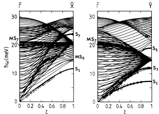
FIG. 9. Calculated phonon-dispersion curves along  $\bar{\Gamma}\bar{X}$  and  $\bar{\Gamma}\bar{Y}$  as in Fig. 7, but with modified force constants in the surface region (Tables I and II).
