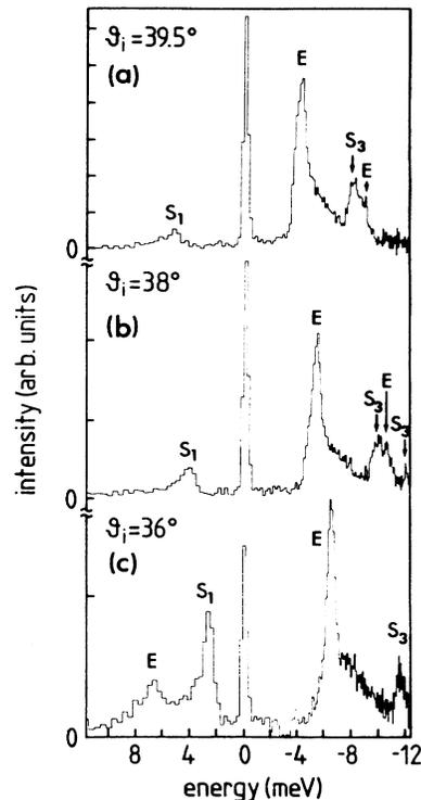
FIG. 4. He-scattering spectra as in Fig. 2, but taken along the  $\bar{\Gamma}\bar{Y}$  direction. The primary He-beam energy was 18.3 meV in all three spectra.
