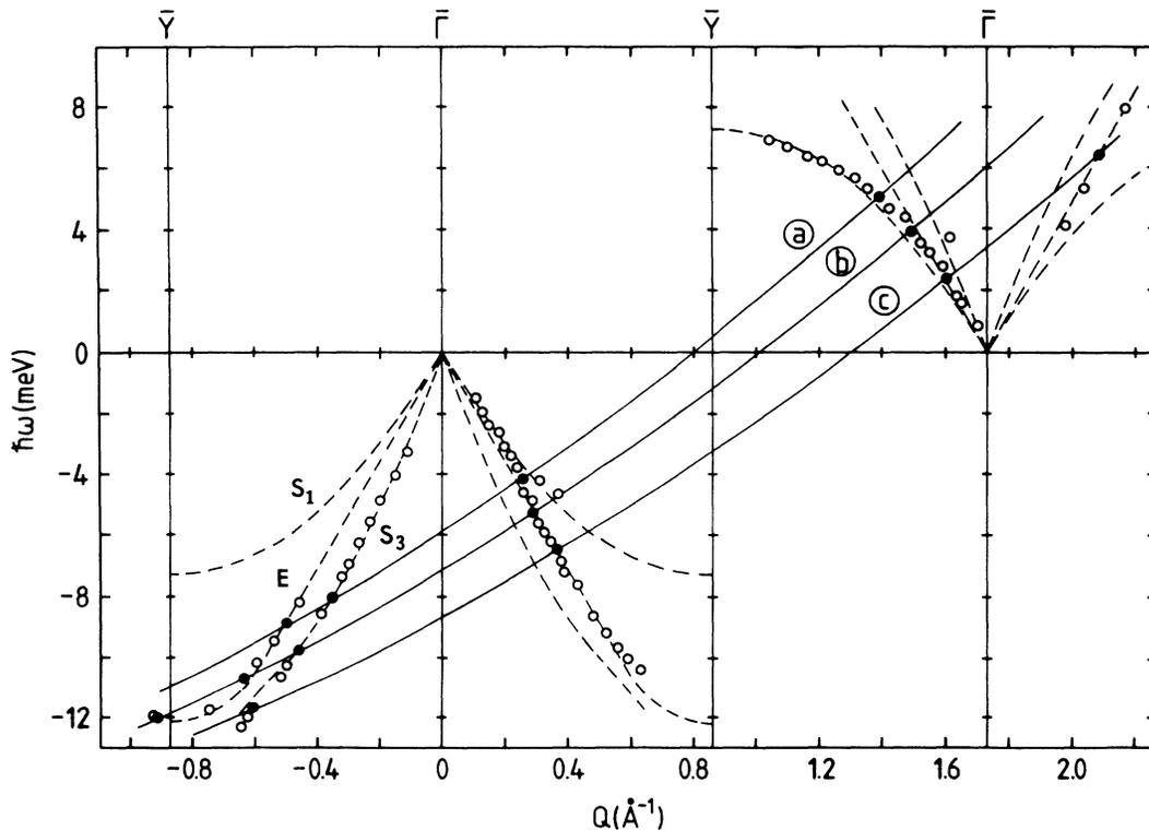
FIG. 6. Same data set as in Fig. 5, but plotted in an *extended* zone scheme, with the actually measured  $Q$  values. The solid lines (a), (b), and (c) are the scan curves [Eq. (1)] corresponding to the scattering conditions in Fig. 4 ( $E_i = 18.3$  meV and  $\theta_i = 39.5^\circ$ ,  $38^\circ$ , and  $36^\circ$ , respectively). The dashed lines through the data points are calculated from a dynamical model fitted to the scattering data (see Sec. III).
