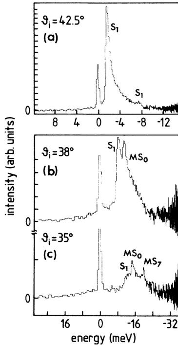
FIG. 2. He time-of-flight spectra taken along the  $\bar{\Gamma}\bar{X}$  direction converted to an energy scale (negative values indicate phonon creation, positive values phonon annihilation). The primary He-beam energy was 18.3 meV (a) and 39.6 meV (b) and (c), respectively. The increase of the noise at higher phonon-loss energies is a feature of the conversion from the time of flight to the energy scale. The phonon peak labels are explained in Secs. III and IV.
