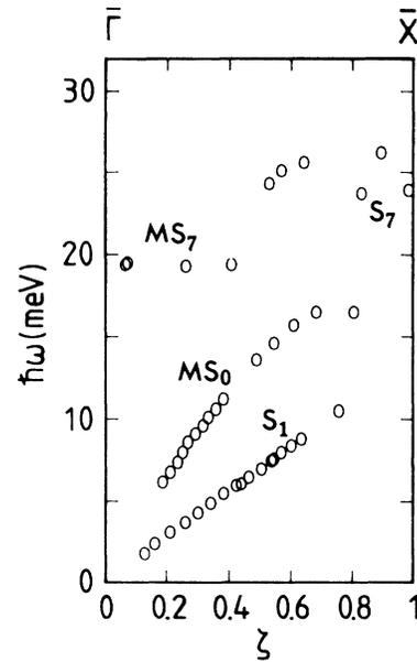
FIG. 3. Experimental data points along the  $\bar{\Gamma}\bar{X}$  direction, plotted in a reduced zone scheme.  $\zeta$  denotes the reduced wave vector defined through  $\zeta = Q/Q_{BZ}(\bar{X})$ , with  $Q_{BZ}(\bar{X}) = 1.23 \text{ \AA}^{-1}$ .
