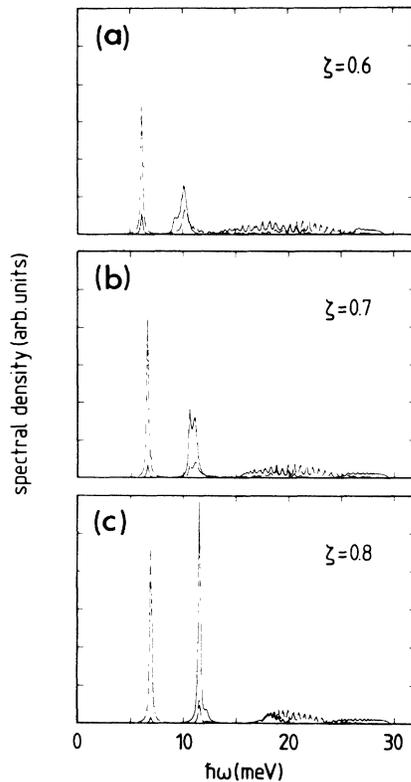
FIG. 10. Spectral density of states for three different reduced wave vectors  $\zeta$  along  $\bar{\Gamma}\bar{Y}$ . Only sagittally polarized modes are shown; the dashed line corresponding to longitudinal polarization, the full line to transverse ( $z$ ) polarization. The calculation was performed with the best fit force constants of Tables I and II, using a 60-layer-thick (110) slab crystal.
