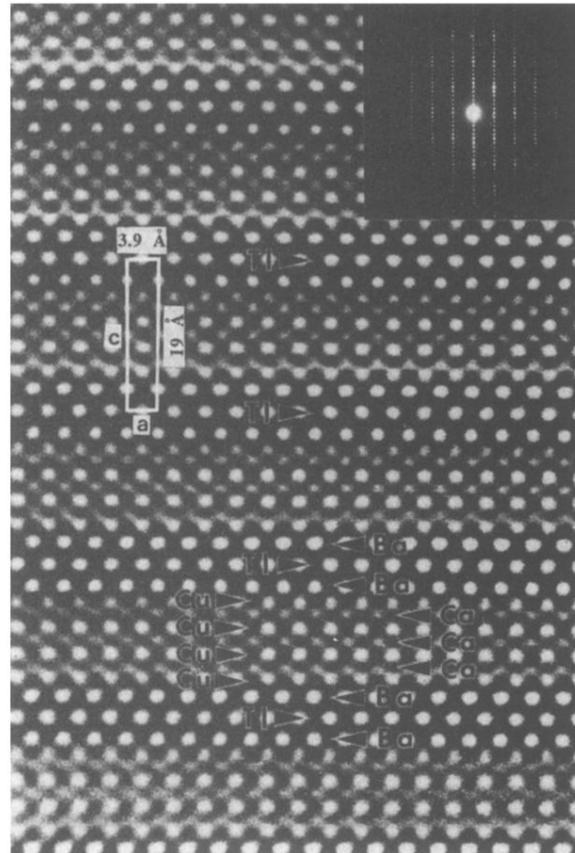
FIG. 2. The electron diffraction pattern and the lattice image of the [010] zone of a  $\text{TlBa}_2\text{Ca}_3\text{Cu}_4\text{O}_{11}$  crystal, which gives a simple tetragonal lattice with lattice constants of  $a = 3.9 \text{ \AA}$  and  $c = 19 \text{ \AA}$ . Each component atom is observed.
