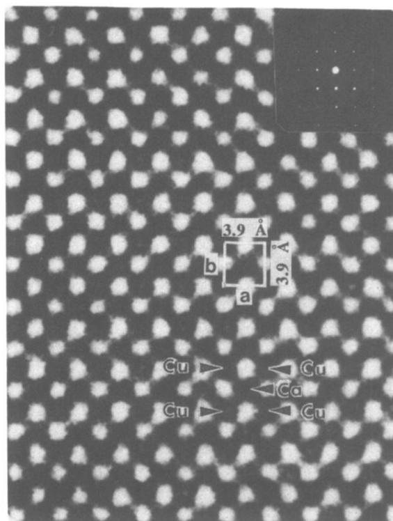
FIG. 1. The electron diffraction pattern and the lattice image of the [001] zone of a  $\text{TlBa}_2\text{Ca}_3\text{Cu}_4\text{O}_{11}$  crystal, which gives a simple square lattice of  $a=b=3.9 \text{ \AA}$ .
