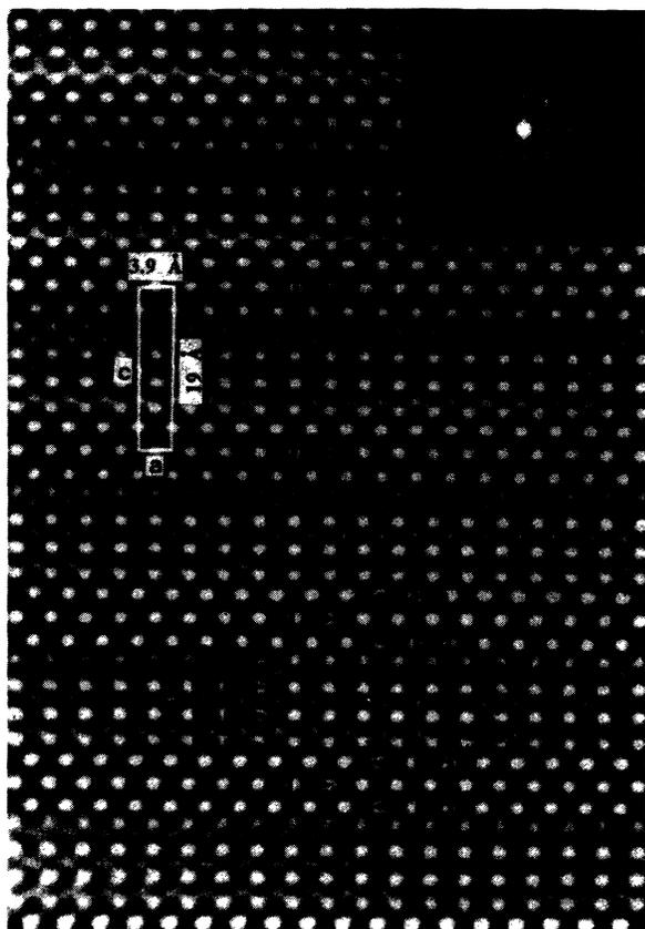
FIG. 2. The electron diffraction pattern and the lattice image of the [010] zone of a  $\text{TlBa}_2\text{Ca}_3\text{Cu}_4\text{O}_{11}$  crystal, which gives a simple tetragonal lattice with lattice constants of  $a = 3.9 \text{ \AA}$  and  $c = 19 \text{ \AA}$ . Each component atom is observed.
