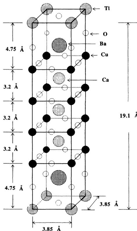
FIG. 3. The lattice structure of a  $\text{TlBa}_2\text{Ca}_3\text{Cu}_4\text{O}_{11}$  crystal with a space group of  $P4/mmm$  and with lattice constants of  $a = b = 3.85 \text{ \AA}$  and  $c = 19.1 \text{ \AA}$ .
