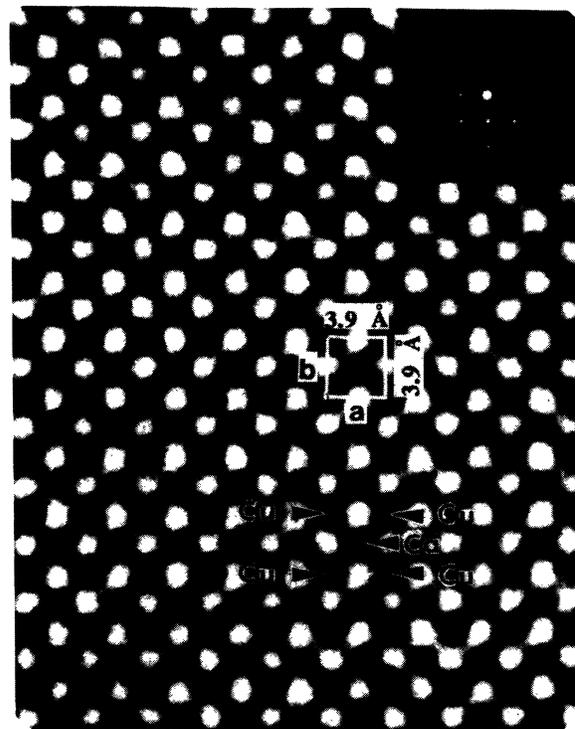
FIG. 1. The electron diffraction pattern and the lattice image of the [001] zone of a  $\text{TlBa}_2\text{Ca}_3\text{Cu}_4\text{O}_{11}$  crystal, which gives a simple square lattice of  $a=b=3.9 \text{ \AA}$ .
