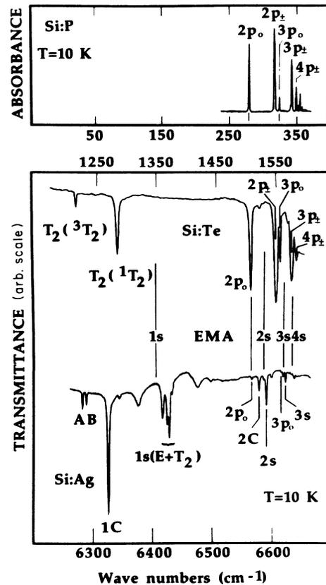
FIG. 3. Comparison between the Ag spectrum and the spectra obtained for the P donor and the neutral Te donor. The energy scales are chosen such that positions of the  $2p_0$  lines coincide. The EMA values for different  $ns$  states are obtained from theory.
