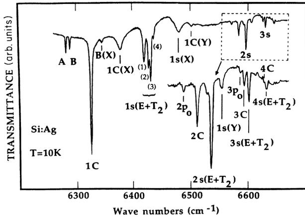
FIG. 2. Transmission spectrum of Ag-doped silicon. For the assignment of the lines see text.
