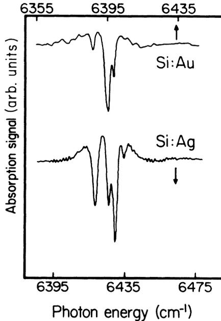
FIG. 4. Comparison of the  $1s(A_1)$ - $1s(E+T_2)$  lines for the Ag and Au donor.
