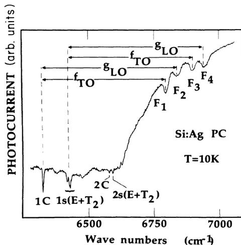
FIG. 5. PTIS spectrum of the Ag donor showing excitation lines due to bound-to-bound transitions and direct excitations to the electronic continuum as well as phonon-assisted Fano resonances. The phonons involved in the resonances are indicated.
