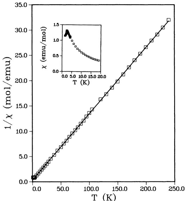
FIG. 1. The reciprocal of molar susceptibility  $\chi$  of  $\text{Gd}_1\text{Ba}_2\text{Cu}_3\text{O}_{6.05}$  vs temperature  $T$ . Inset:  $\chi$  vs  $T$ , showing the antiferromagnetic transition of the Gd system.
