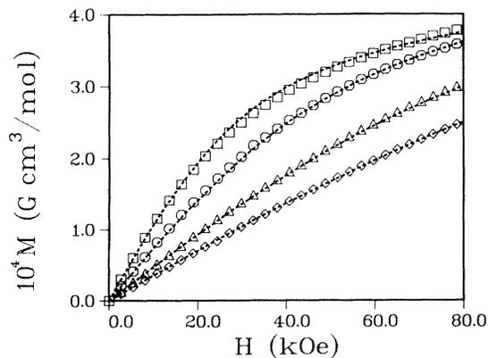
FIG. 7. The molar magnetization of oxygen-depleted Ho 1:2:3 at 4.5 K ( $\square$ ); 10 K ( $\circ$ ); 20 K ( $\triangle$ ); and 30 K ( $\diamond$ ). Broken lines are model fits (see text).
