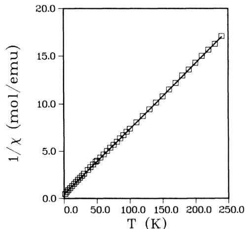
FIG. 4. The reciprocal molar susceptibility of  $\text{Dy}_1\text{Ba}_2\text{Cu}_3\text{O}_{6.95}$  vs temperature.
