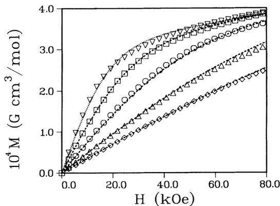
FIG. 5. The molar magnetization of oxygen-depleted Dy 1:2:3 vs field  $H$  at 1.5 K ( $\nabla$ ); 4.2 K ( $\square$ ); 10.0 K ( $\circ$ ); 20.0 K ( $\triangle$ ); and 30.0 K ( $\diamond$ ). The broken lines are calculated using Eq. (3) in the text.
