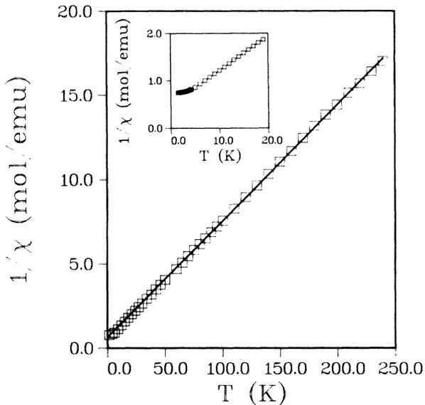
FIG. 6. The inverse molar susceptibility of  $\text{Ho}_1\text{Ba}_2\text{Cu}_3\text{O}_{6.05}$ . Inset:  $1/\chi$  vs  $T$  at low temperature.
