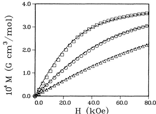
FIG. 3. The magnetization per mole of oxygen-depleted Gd 1:2:3 compound vs applied magnetic field  $H$ , at temperatures of 4.5 K ( $\square$ ); 10.0 K ( $\circ$ ); and 20.0 K ( $\triangle$ ). The broken lines are model fits using Eq. (2).
