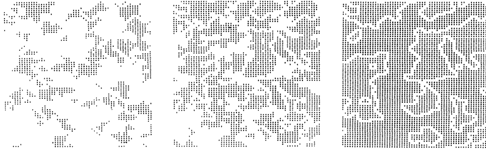
FIG. 13. Computer simulations of c(2 \times 2) island formation for chemisorption with Eden rates k_i = 200k_0 , i \geq 1 , for x = \Theta/\Theta^* = \frac{1}{3}, \frac{2}{3}, 1 . X , Y , and \circ as in Fig. 9.
