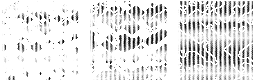
FIG. 9. Computer simulation of c(2 \times 2) island formation for chemisorption with multiplicative rates, k_i \propto 40^i , for x = \Theta/\Theta^* = \frac{1}{3}, \frac{2}{3}, 1 . X and Y denote filled sites in domains of different phase; \circ denoting empty sites are only shown within c(2 \times 2) domains for contrast.
