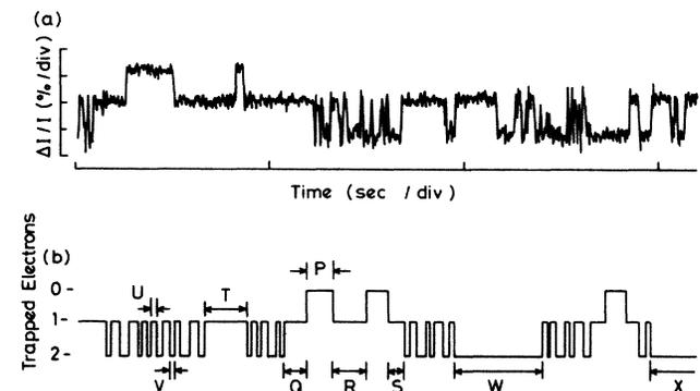
FIG. 3. (a) Complex RTS generated by a single defect which shows one- and two-electron capture.  $T = 290$  K,  $V_G = 0.6$  V,  $V_D = 20$  mV, and  $I_D = 195$  pA. (b) Schematic RTS showing all the features which were observed for this defect.
