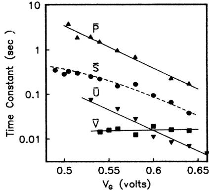
FIG. 4. Gate-voltage dependence of representative times  $\bar{P}$ ,  $\bar{S}$ ,  $\bar{U}$ , and  $\bar{V}$  from the RTS shown in Fig. 3. The solid lines are regression lines and the dashed line is a fit assuming simple competition between emission and capture in the  $\theta_1$  state.
