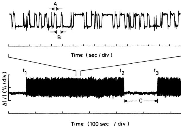
FIG. 1. Fluctuations in current vs time showing a rapidly switching RTS modulated by an envelope of the same amplitude. The upper trace is an expansion of part of the lower trace.  $V_G = 1$  V,  $V_D = 10$  mV,  $I_D = 10.3$  nA, and  $T = 293$  K.
