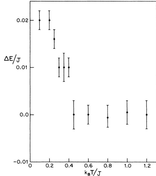
FIG. 4. Temperature dependence of  $\Delta E/J$ , the difference in energy per spin between zero-field-cooled and field-cooled runs for  $\langle f \rangle = 7$ .
