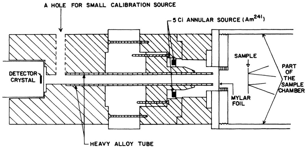
FIG. 1. Schematic diagram of the source-collimator assembly.
