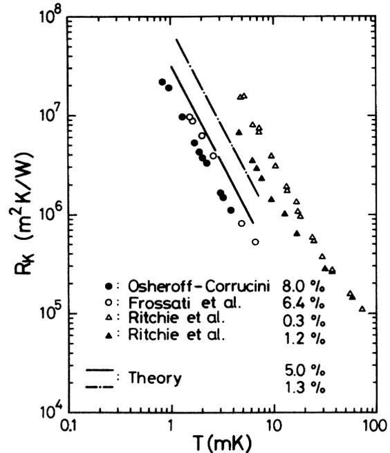
FIG. 2. The Kapitza resistance  $R_K$  of dilute  $^3\text{He}$ - $^4\text{He}$  solutions as a function of temperature. Data are taken from Refs. 4-6. Solid lines are the theoretical ones calculated from Eq. (8). The lower line is for 5.0% solution, and the upper one is for 1.3% solution, respectively.
