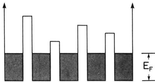
FIG. 1. Conceptual illustration of potential wells for  $^3\text{He}$  quasiparticles confined in small pores 100 Å in diameter. The barriers correspond to the narrow channels.
