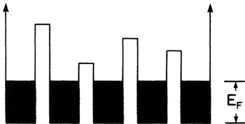
FIG. 1. Conceptual illustration of potential wells for  $^3\text{He}$  quasiparticles confined in small pores 100 Å in diameter. The barriers correspond to the narrow channels.
